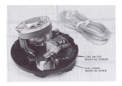
Fig. 5—Removing Line Switch and Dial Mounting Frame
