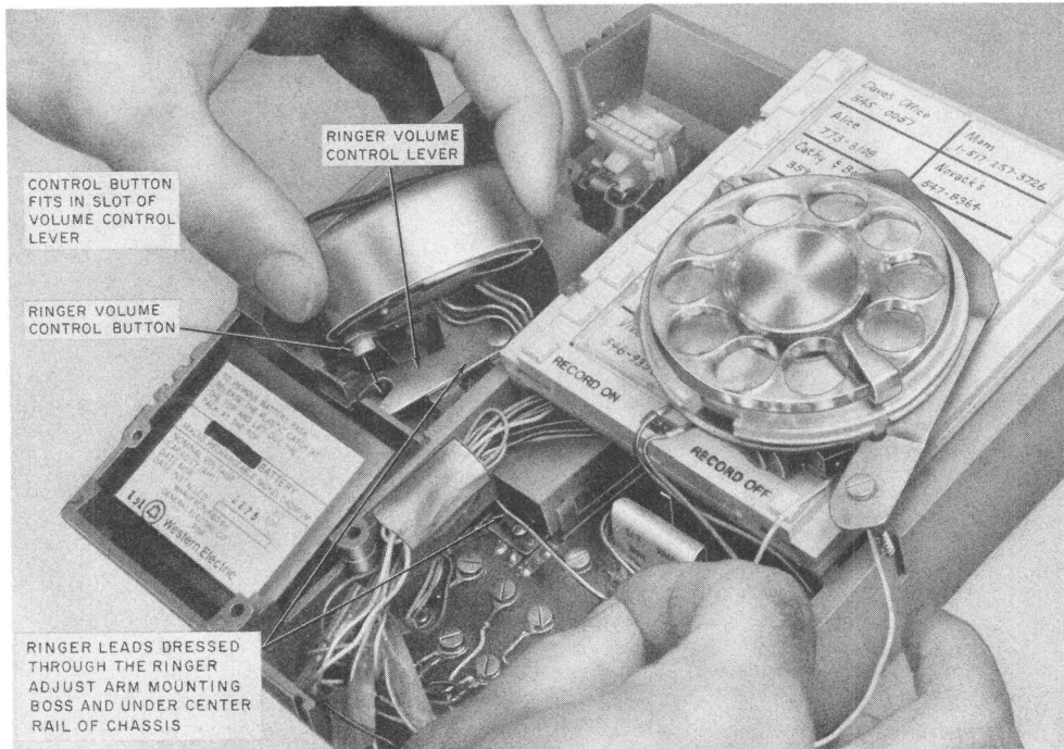
Fig. 10—Ringer Being Installed in 960A01M Chassis With Dial Rotated Onto Memory and Shield Removed
