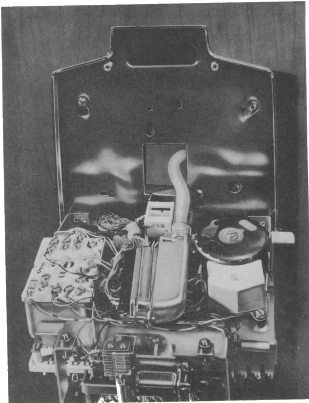
Fig. 10—Connector Cable and D-180375 Kit of Parts
