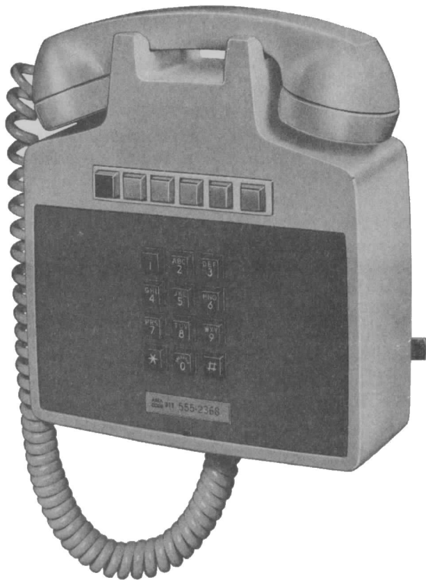
Fig. 6—2851-Type Telephone Set, Assembled Station
