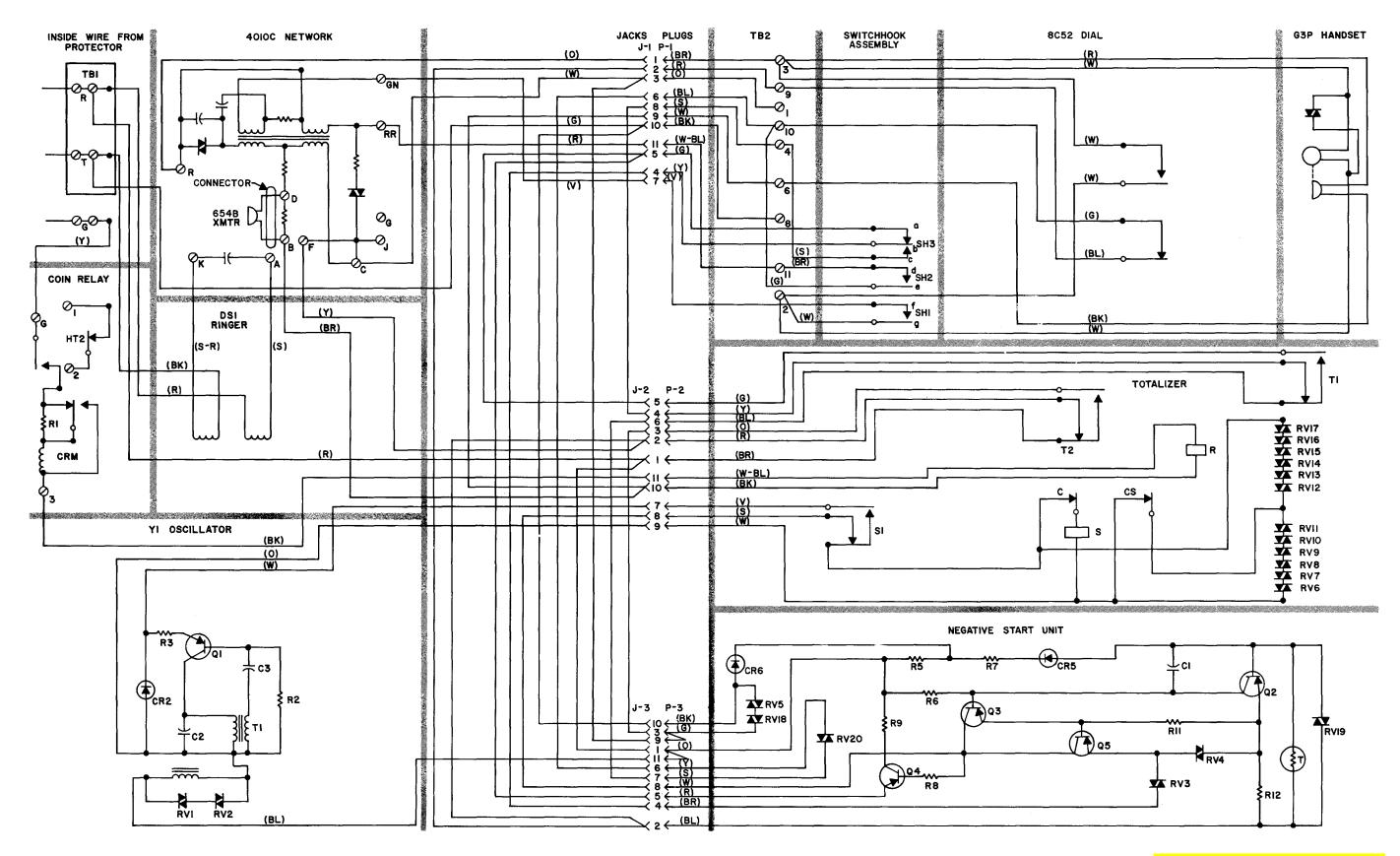
Fig. 1 - IAI and IA2 Coin Telephones, Connecting Diagram
