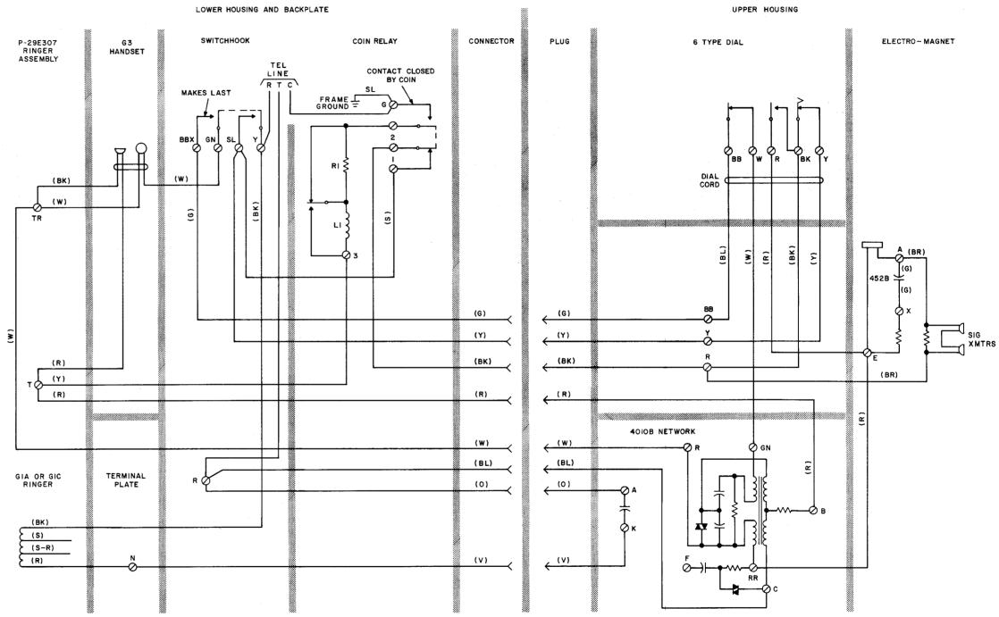
Fig. 1 — 236G Coin Collector Telephone Set — Connections
