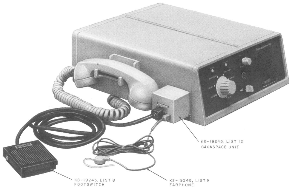
Fig. 26—KS-19245 Type Telephone Answering Set—With Accessories
