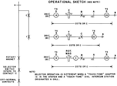
Fig. 2—Basic Operation of Selector Circuit Using Rotary Dial
