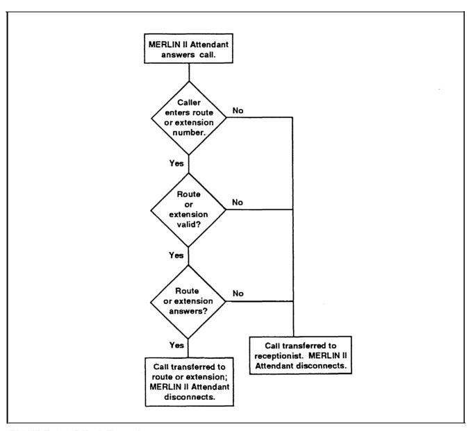
FIGURE 2-1 Blind Transfer process.
