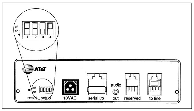
FIGURE 1-3 Setup Switch Positions for Installing Unit.
