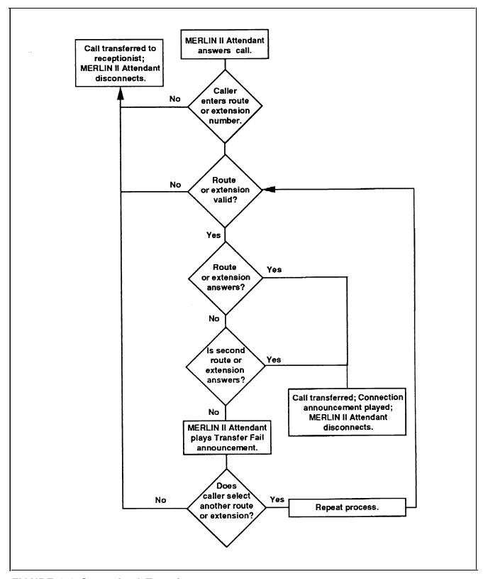
FIGURE 2-2 Supervised Transfer process.
