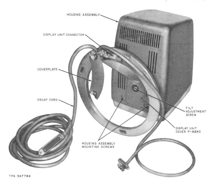
♦ Fig. 19—Bottom View of 1A Display Unit 4
