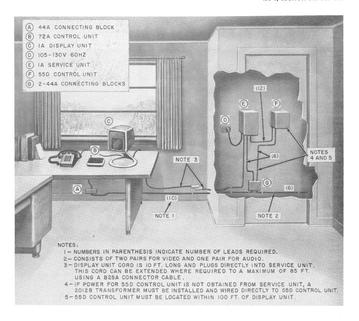
Fig. 9—Typical Installation of Single Line Station
