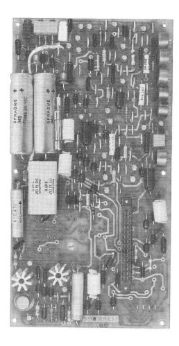
Fig. 17—939B Cable Equalizer
