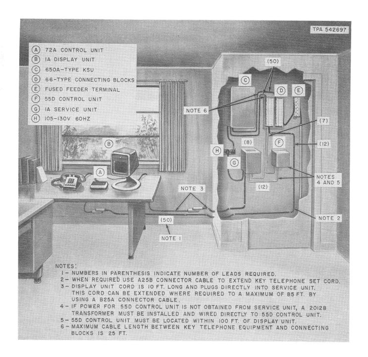
Fig. 10—Typical Installation of Key Telephone Station
