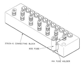
Fig. 13—Method of Fusing for PICTUREPHONE Equalizer
