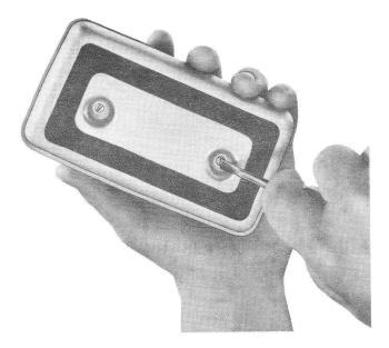
Fig. 20—Removing Housing and Panel Assembly
