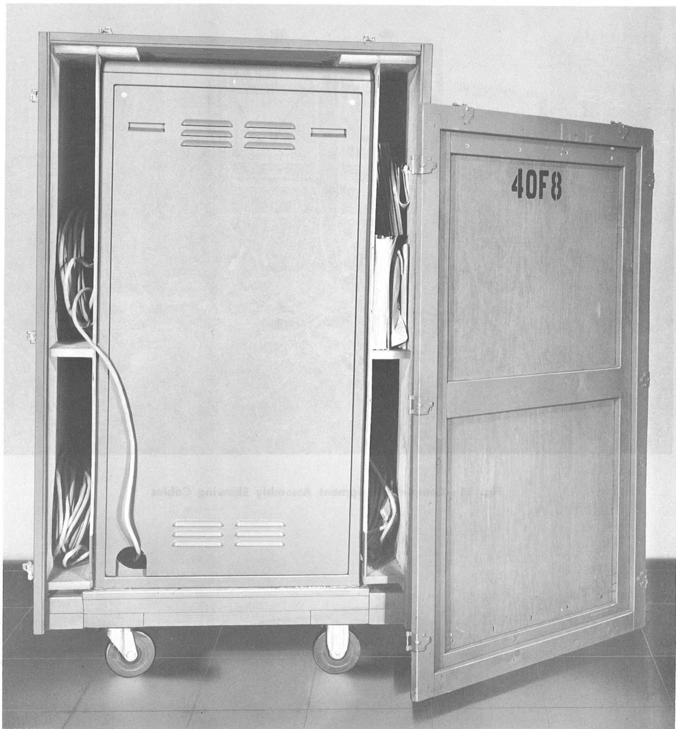
Fig. 10—Cabinet No. 4 Showing Cable and Drawing Storage
