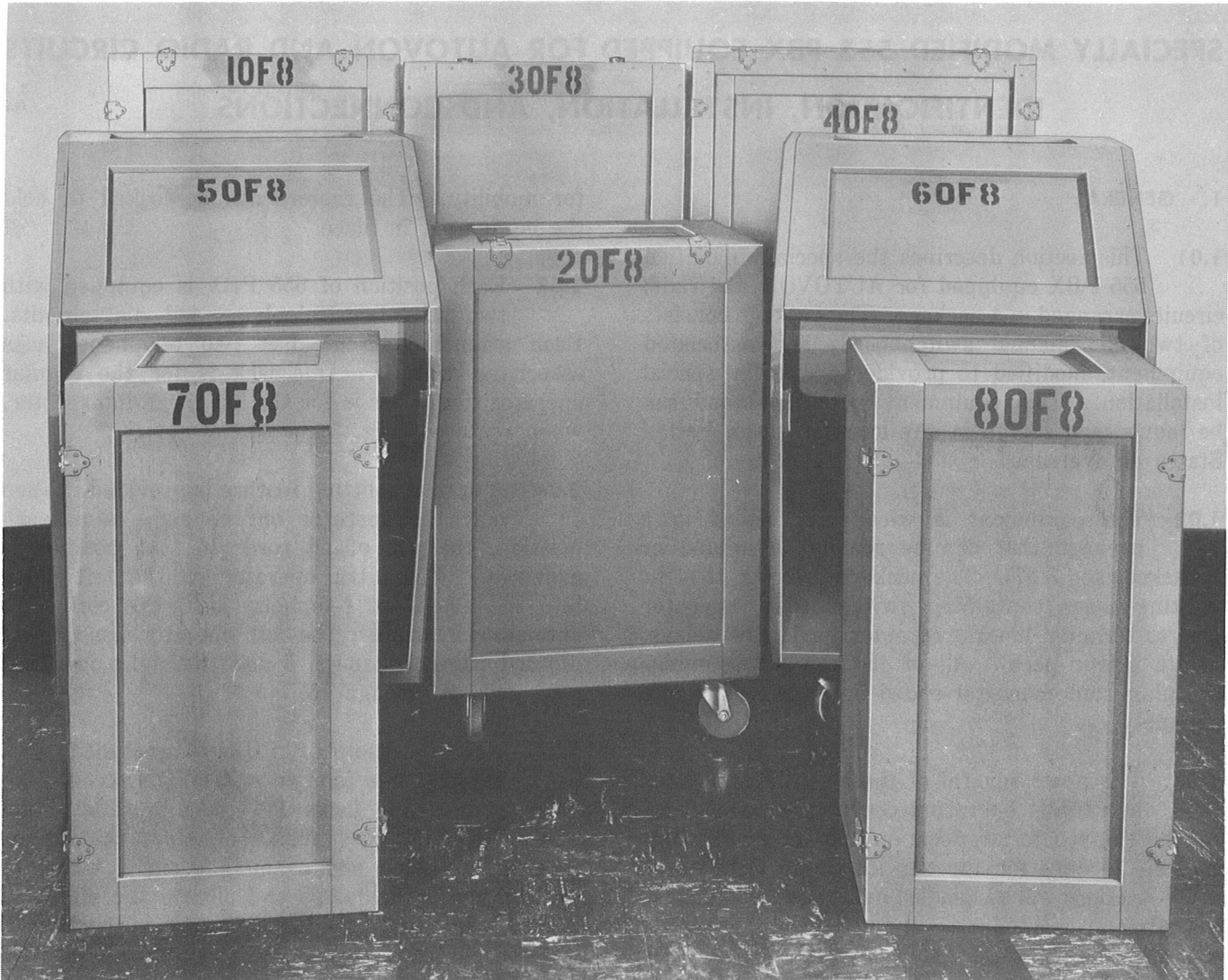
Fig. 1—Specially Modified 555 PBX Equipment in Crates
