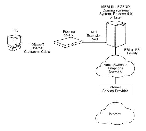
Figure 1. Diagram of a Pipeline 25-Px with a MERLIN LEGEND Communications System.
