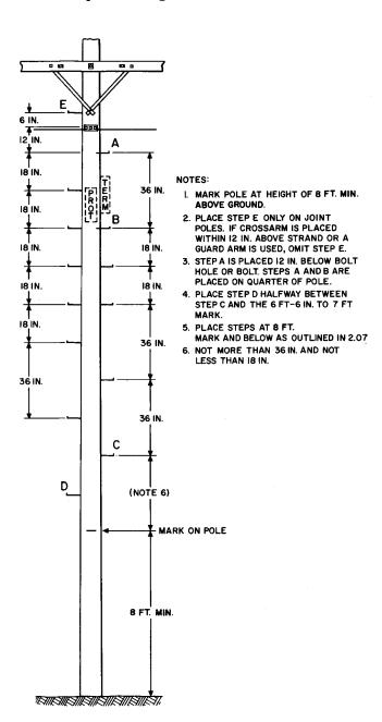
Fig. 11—Terminal on Face or Back
