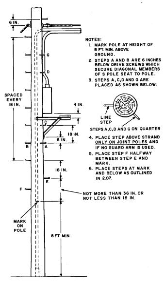
Fig. 16—Steps for Cross-Connect Terminals
