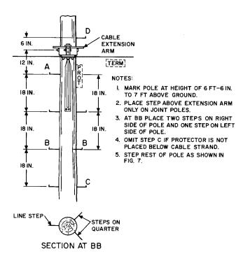
Fig. 9—Extension Arm With Terminal on Right
