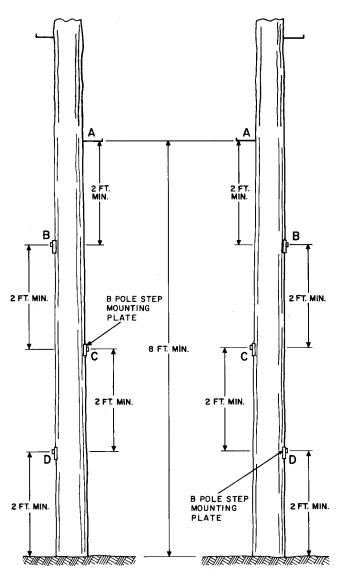
Fig. 6—B Pole Step Spacing
