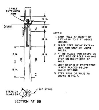
Fig. 8-Extension Arm With Terminal on Left
