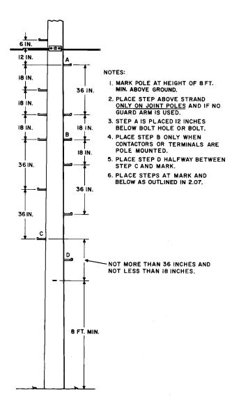
Fig. 17—Steps on Poles Supporting Equipment
