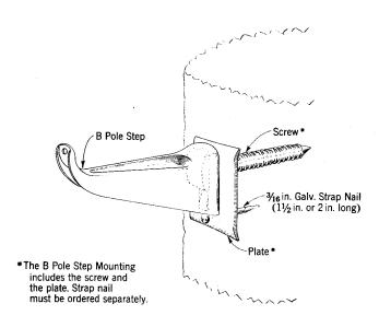
Fig. 5-Mounted B Pole Step
