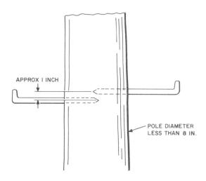
Fig. 3—Double Step in Small Diameter Pole
