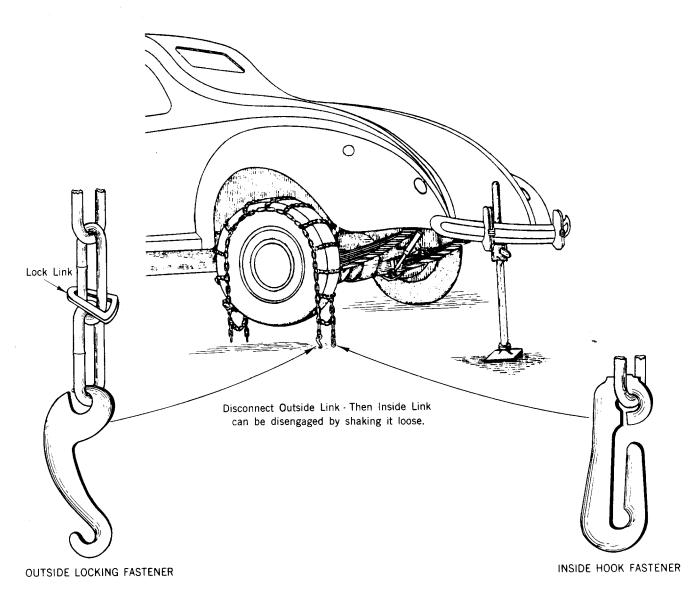
ATTACHING OR REMOVING ROLLER GRIP TIRE CHAIN
