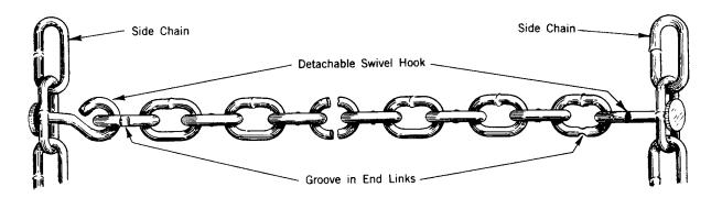
CROSS CHAIN AND SWIVEL HOOK ASSEMBLED TO SIDE CHAINS
