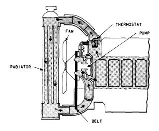
Fig. 2—Coolant Circulation Path
