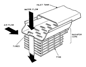
Fig. 3—Typical Radiator Construction
