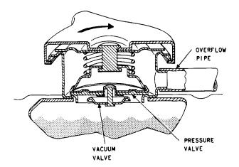
Fig. 4—Vented Pressure Cap
