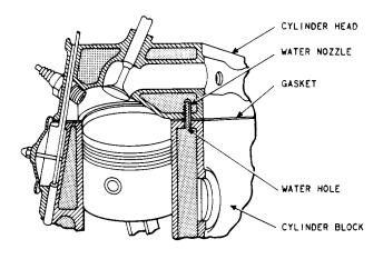
Fig. 1—Coolant Passages in Water Jacket
