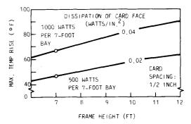
Fig. 2—Temperature Rise in Free Convection for Equipment of Different Height
