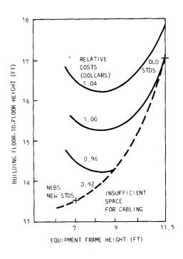
Fig. 1—Relative Costs for Equipment-Building Systems
