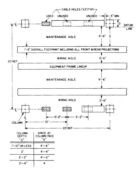
Fig. 3—Typical Standard Floor Plan for 18-Inch Deep Frames
