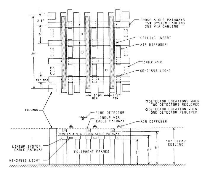
Fig. 11—Cable Pathways Plan for 12-Inch Deep Frame Areas
