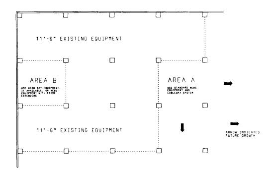
Fig. 4—NEBS Equipment in Non-NEBS Space Presently Occupied By Highbay Equipment
