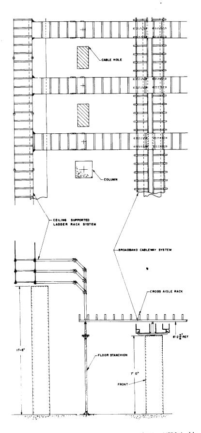
Fig. 16—Interface of NEBS Broadband Cableway System with Non-NEBS Ladder Rack System
