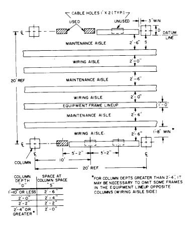
Fig. 2—Typical Standard Floor Plan for Principal Depth 12-Inch Frame
