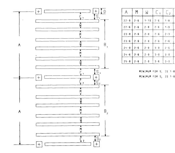
Fig. 7—Recommended Floor Plans for Principal Depth 12-Inch Frames for Column Spacings Between 22 Foot, 0 Inch and 25 Foot, 0 Inch
