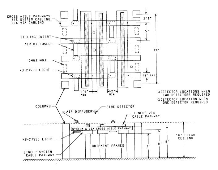
Fig. 12—Cable Pathways Plan for 18-Inch Deep Frame Areas
