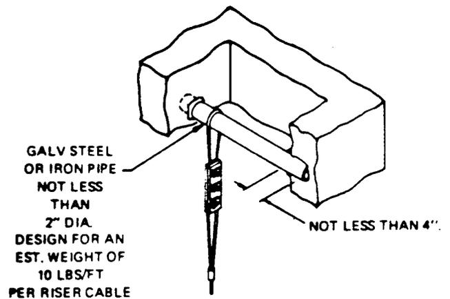
Fig. 8—Cable Support at Ceiling Level
