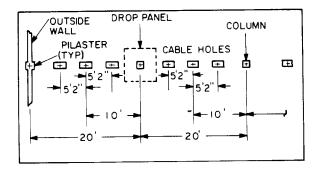
Fig. 10—Plan for Plugged Cable Openings for Future Use
