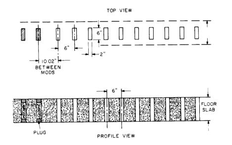
Fig. 6—Rectangular Frame—Opening—Pattern Modular Protector Frames
