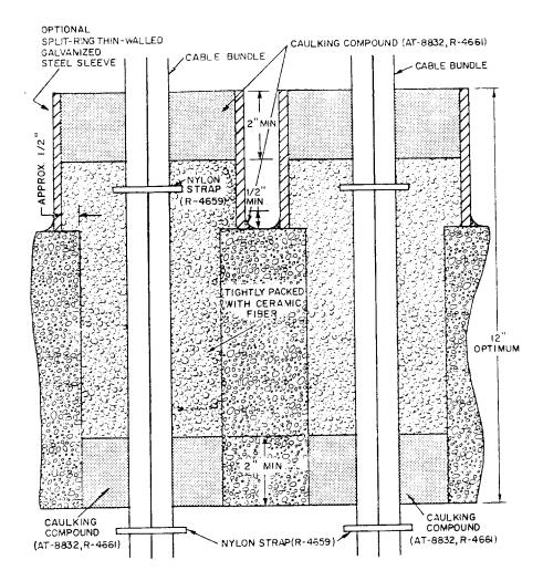
Fig. 9—Recommended Fire-Stopping Configuration for 2- by 6-Inch and 4- by 6-Inch Cable Holes
