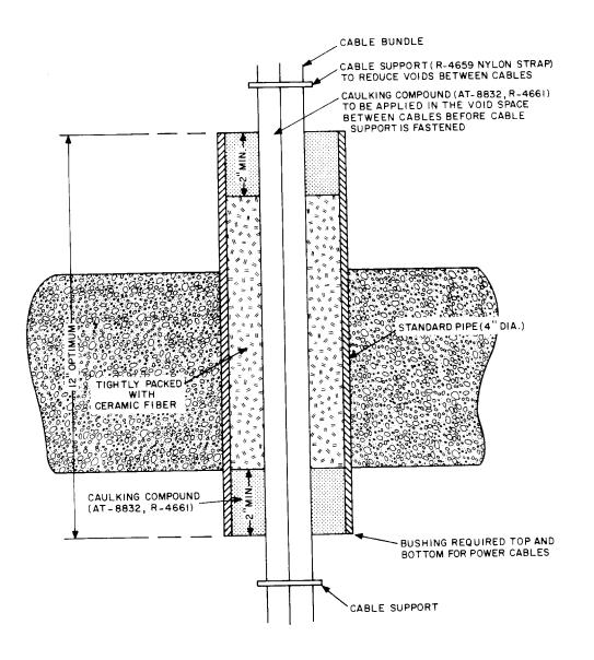
Fig. 3—Fire-Stopping Configuration for Circular Cable Openings
