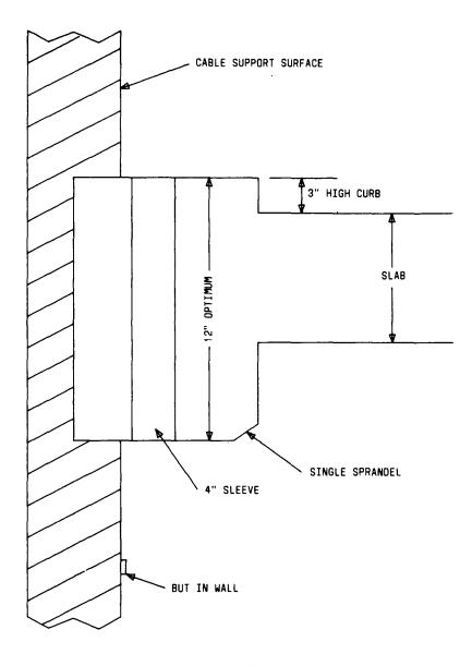
Fig. 1—Typically Upper Floor Riser Construction
