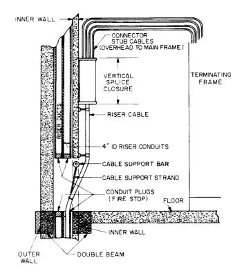
Fig. 4—Riser Cable System
