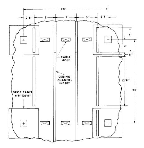
Fig. 5—Section of Equipment Room Showing Location of Channel Inserts (UNISTRUT) for Each 20' imes 20' Bay
