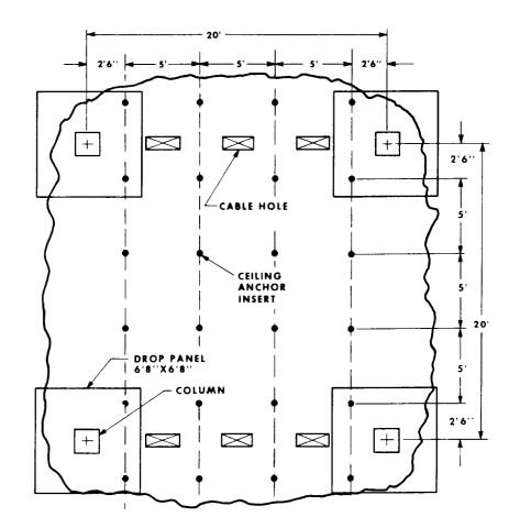
Fig. 4—Section of Equipment Room, Showing Location of Anchors
