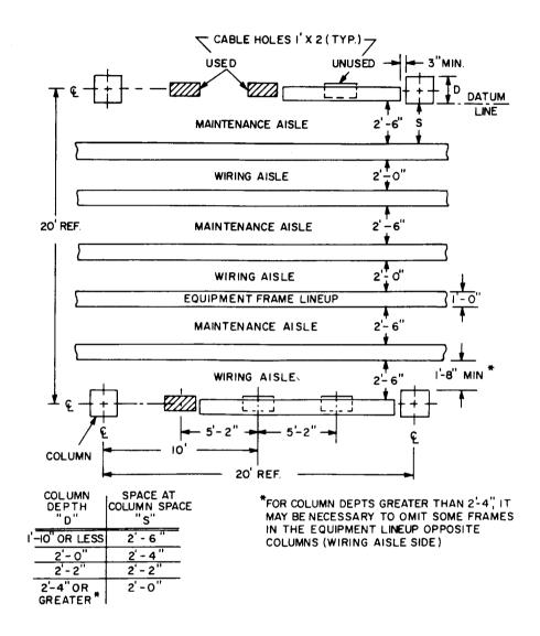
Fig. 1—NEBS Standard Floor Plan for Principal Depth 12-Inch Frame
