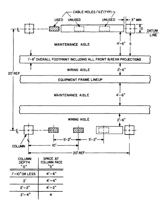
Fig. 2—NEBS Standard Floor Plan for 18-Inch Deep Frames
