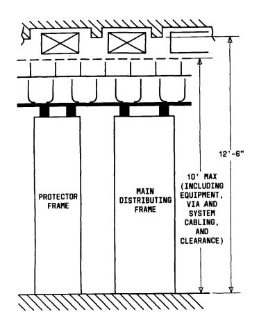
Fig. 4—Typical Distributing Frame Area
