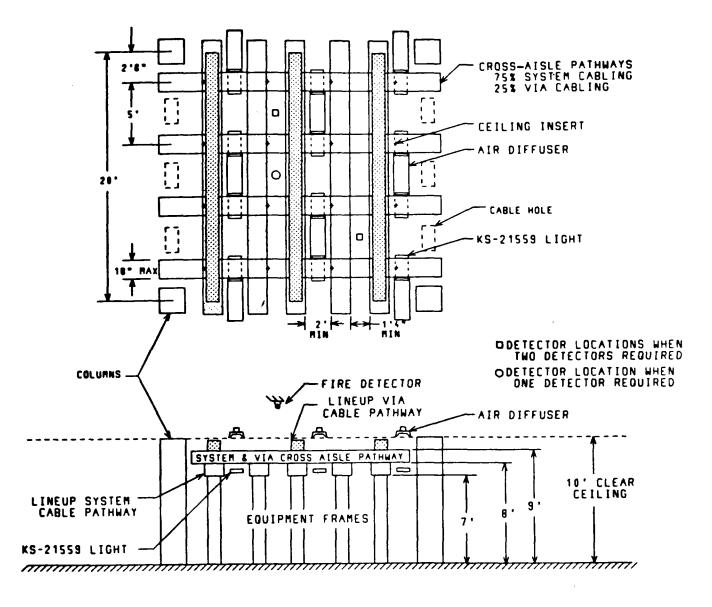
Fig. 2—Cable Pathways Plan for 7- to 10-Foot Space
