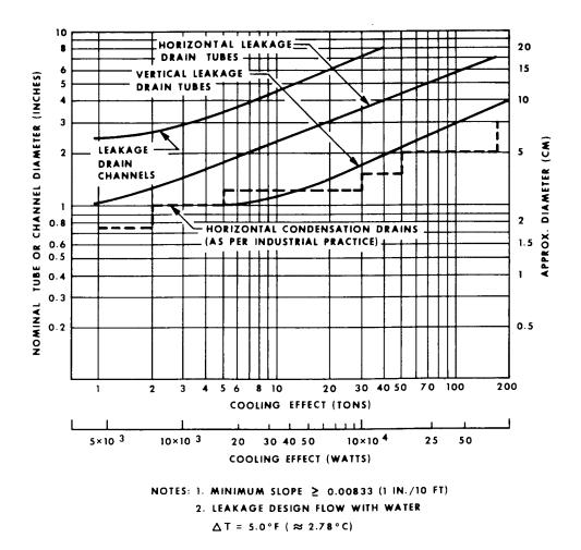
Fig. 3—Recommended Drain Tubes and Channels for Process Coolers and Chillers
