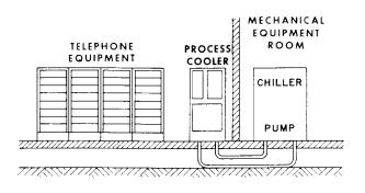
Fig. 2—Vertical System—Process Coolers on Each Floor, All Fed by a Single Chiller
