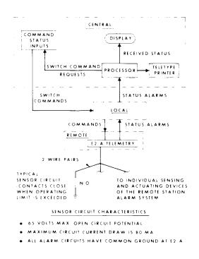
Fig. 2—Telemetry Alarm System Block Diagram
