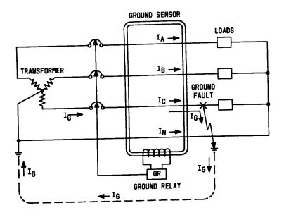
NORMAL LOADS -  $I_A + I_B + I_C + I_N = 0$ Ground Fault Path  $\rightarrow$  relay operates
