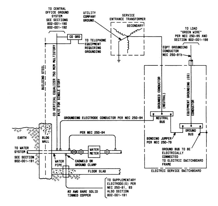
Fig. 1—Typical Grounding Schematic
