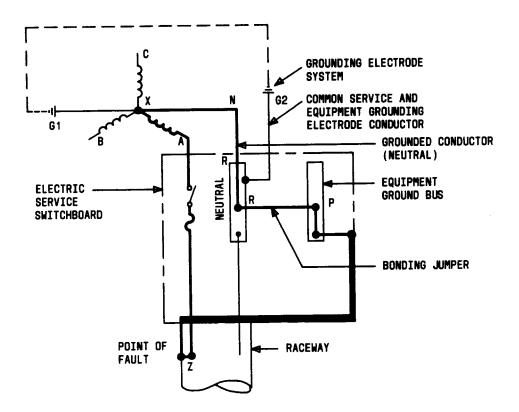
Fig. 2--Simplified Service and Equipment Grounding Schematic
