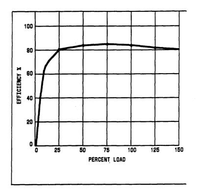
Fig. 1—Efficiency of Typical 3-Phase Motor
