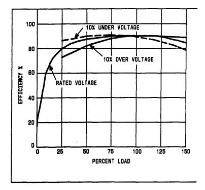
Fig. 2—Efficiency Sensitivity of Typical 3-Phase Motor
