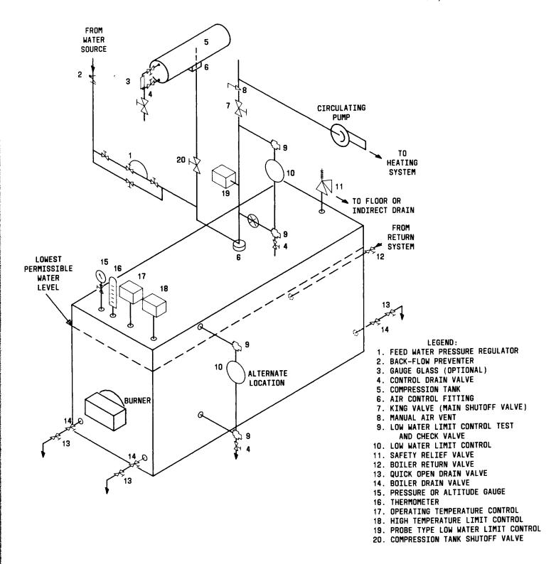
Fig. 1—Hot Water Boiler
