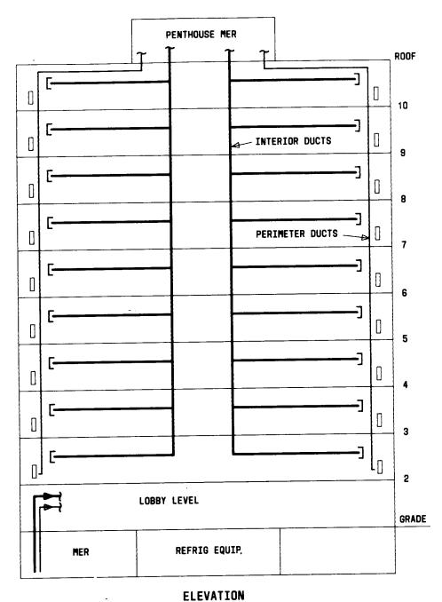
Fig. 6—High-Rise Office Building (Up to Ten Floors) (Sheet 1 of 2)
