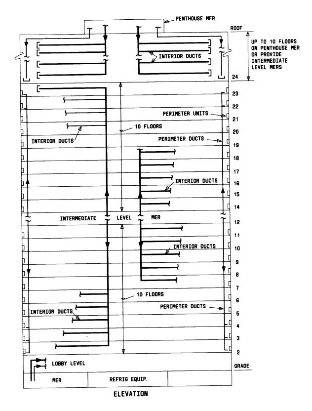
Fig. 7—High-Rise Office Building (Over Ten Floors) (Sheet 1 of 2)
