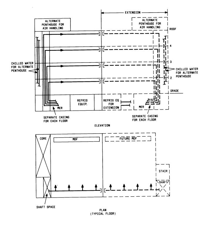
Fig. 4—Acceptable Location for MER in CO Equipment Building (4-Bay Extension) (Sheet 1 of 2)
