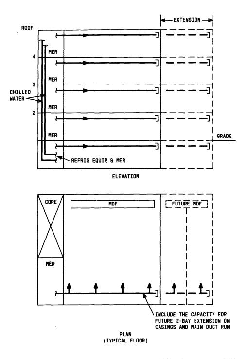
Fig. 1—Preferred Location for MER in CO Equipment Building (2-Bay Extension) (Sheet 1 of 2)
