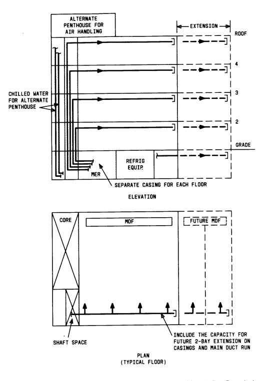
Fig. 3—Acceptable Location for MER in CO Equipment Building (2-Bay Extension) (Sheet 1 of 2)
