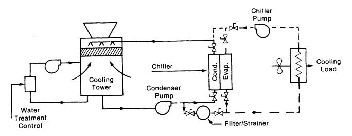
Fig. 10—Filtration or Strainer System
