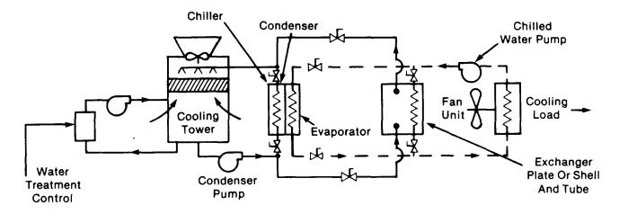
Fig. 11—Cooling Tower and Heat Exchanger
