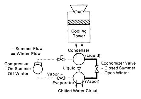
Fig. 8—Chiller Vapor Cycle
