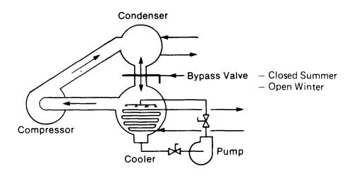
Fig. 9—Pumped Vapor Cycle
