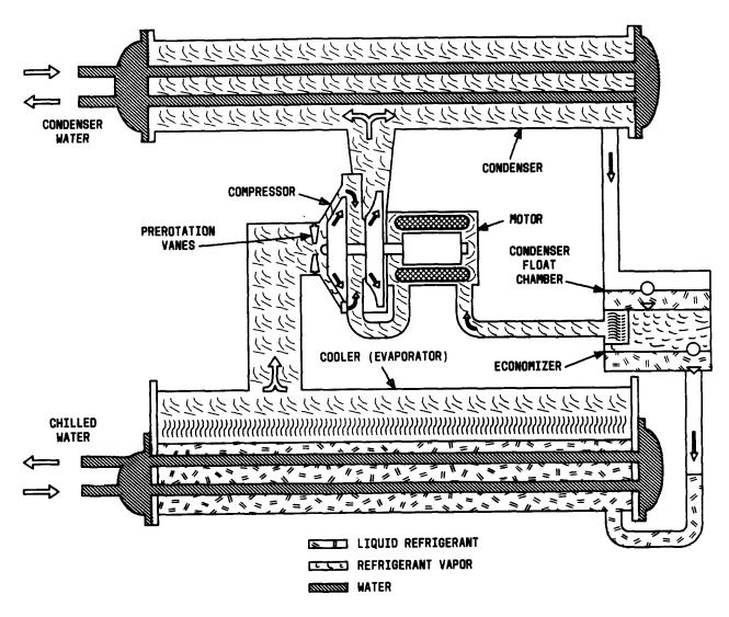
Fig. 2—Refrigeration Cycle Diagram (Carrier Corporation)
