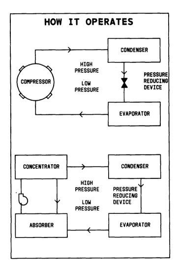
Fig. 3—Comparison of Mechanical Refrigeration Cycle and Absorption Refrigeration Cycle
