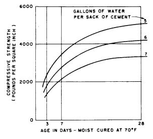
FIG. A NORMAL PORTLAND CEMENT CONCRETE
