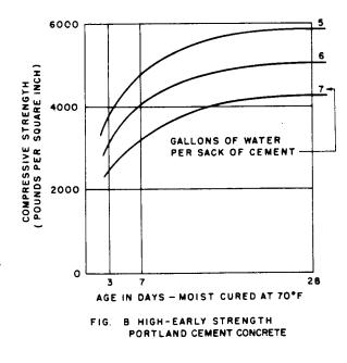
Fig. 4—Compressive Strength Curves
