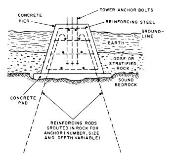
Fig. 3—Typical Foundation in Rock
