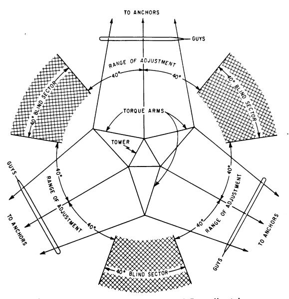
Fig. 2 – Azimuth Limitations for 8 x 12 Foot Reflectors Mounted on B Guyed Towers
