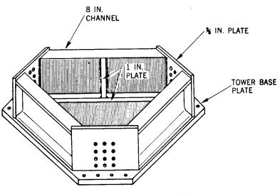
INTERNAL BRACING OF TOWER BASE
