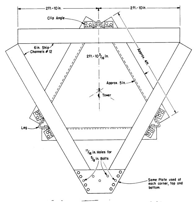
Fig. 11 – Triangular Brace for Attachment of Reflector Backstays
