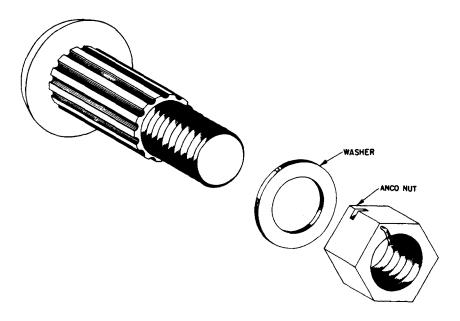
Fig. 2 - Structural Rib Bolt Assembly
