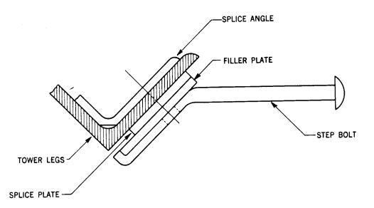
Fig. 13 – Typical Step Bolt at Leg Splice
