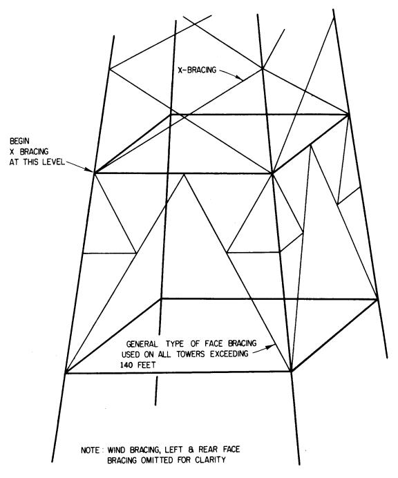
Fig. 10 - Types of Face Bracing
