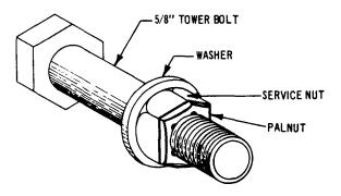
Fig. 4 – Typical Bolt Assembly
