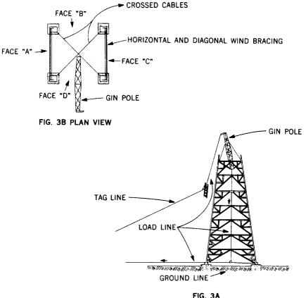
TYPICAL GIN POLE FOR HOISTING TOWER SECTIONS
