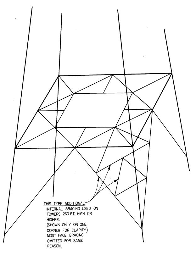
Fig. 6 – Types of Internal Bracing
