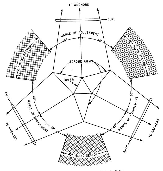
Fig. 2 – Typical Azimuth Limitations of Passive Reflectors Used With E Guyed Towers
