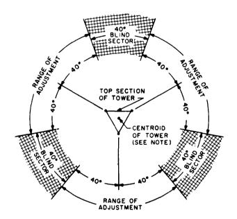
FIG.88. AZIMUTH LIMITATIONS OF KS -16320 -LI 6'X8' REFLECTORS
