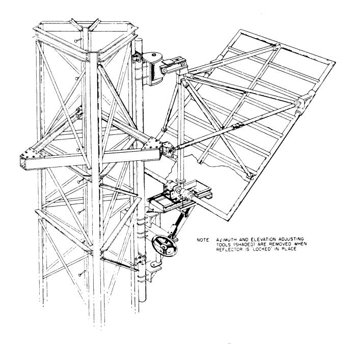
Fig. 5 - Mounted 5- by 8-Foot Reflector
