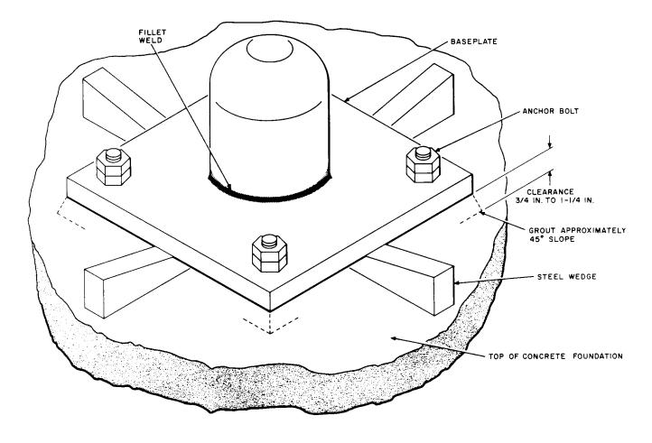
Fig. 1—Installation of Base Plate Assembly
