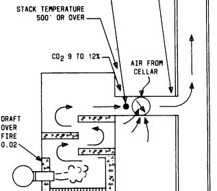
Fig. 12—Draft Control Can Increase Operating Efficiency
