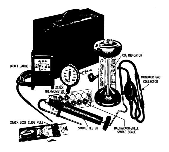
Fig. 1—Combustion Efficiency Testing Kit
