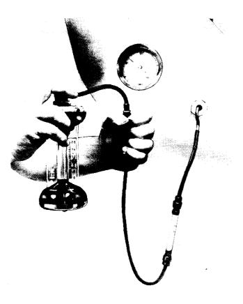
Fig. 6—Taking a Flue Gas Sample
