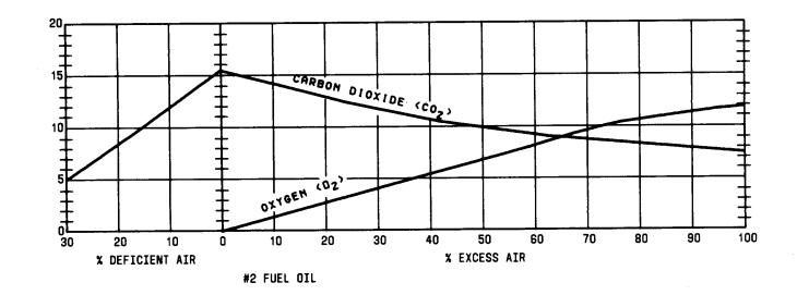
Fig. 9—Percent of Excess Air for Various CO<sub>2</sub> and Oxygen Readings
