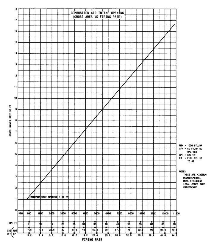
Fig. 16—Combustion Air Intake Opening (Gross Area Versus Firing Rate)
