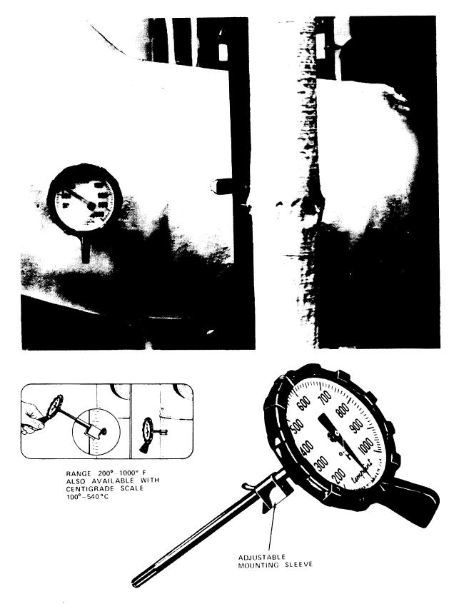
Fig. 3—Testing Stack Temperature
