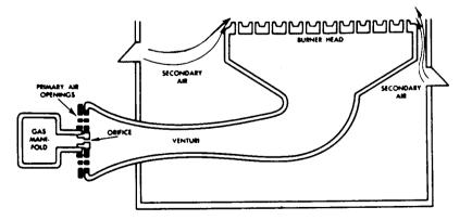
Fig. 14---Typical Atmospheric Burner
