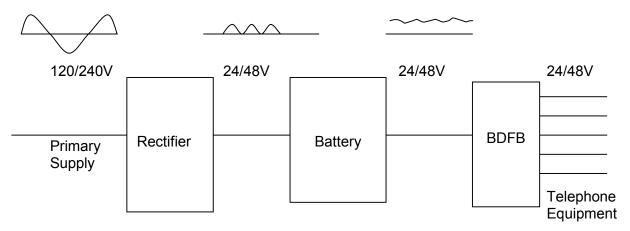
6.03 The office dc power system including standby power sources shall provide protected ac power for network operations support systems installed in the building. The amount of protection provided shall be based on the requirements of the installed system(s) rather than a generic value.
