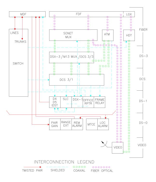
Figure 8-2 - Generic Functionality Of Transport Equipment Network Elements
