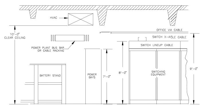
Figure 2-2 - Clear Ceiling - Power And Switching Areas
