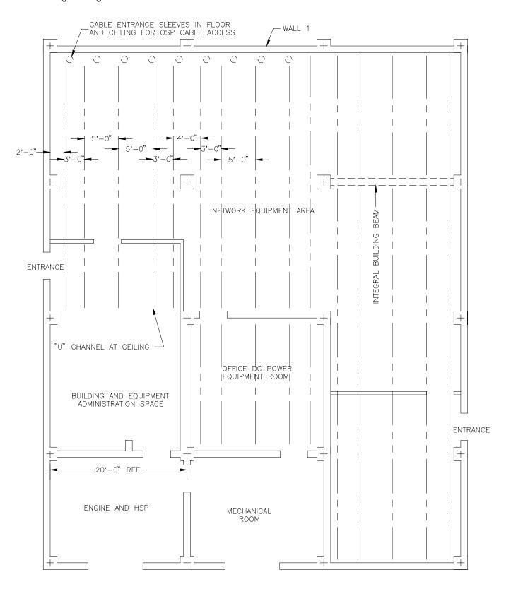
Figure 2-1 - Generic Layout Of Office Superstructure Support Channel
