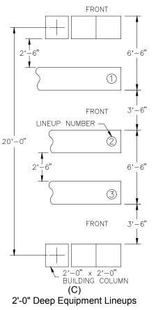
Figure 9-3 Typical Aisle Spaces For 1'-3", 1'-6" and 2'-0" Deep Equipment Lineups
