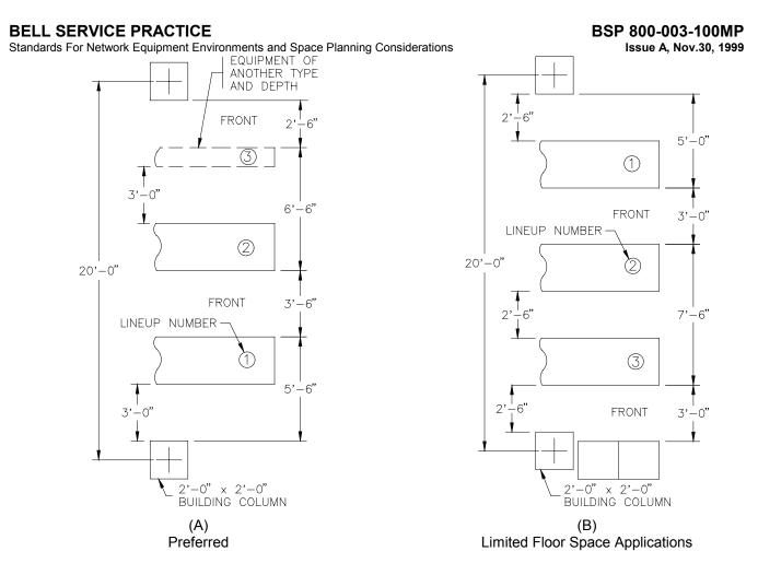
Figure 9-4 Typical Aisle Spaces For 2'-6" Deep Equipment Lineups
