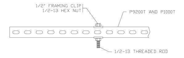
Figure 13 <sup>1</sup>/<sub>2</sub> Inch Hanger Rod
