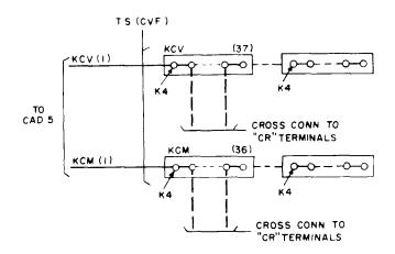
Fig. 14 — Use of K4 to Indicate Right-Hand Terminal Lug of a Group of Terminals Looking at Rear of 236- or Similar-Type Terminal Strip
