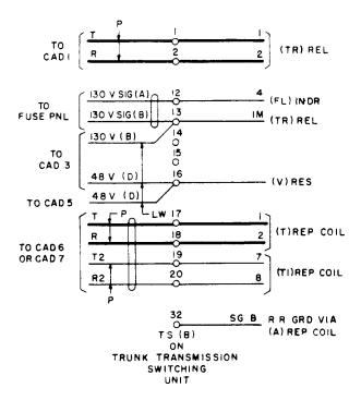
Fig. 20 — Terminal Assignment on 224-Type
