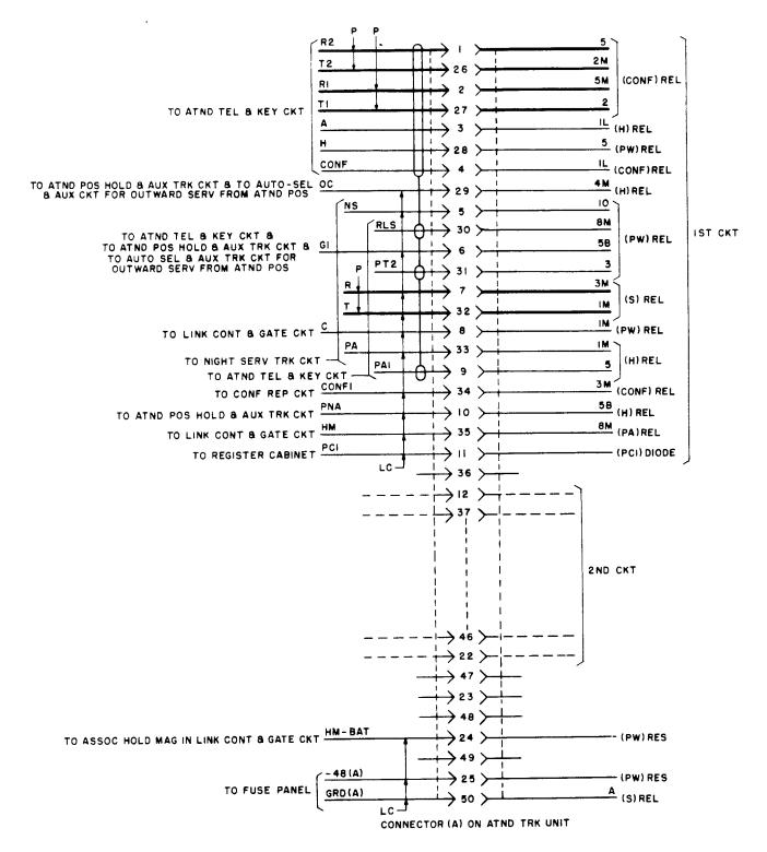
Fig. 22 – Method of Showing Connectors (KS-16785 Plug and KS-16786 Connector shown)
