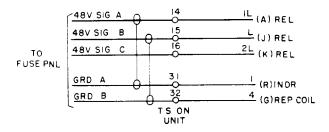
Fig. 27 - Battery and Ground Lead Designations
