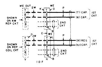
Fig. 23 — Identification Designations on Terminal Strips
