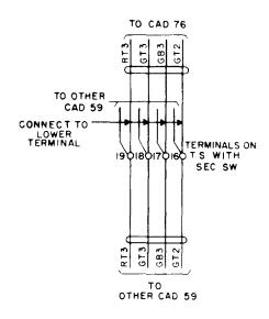
Fig. 13 – Method of Showing Connection to 216-Type Terminal Strip
