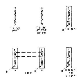
Fig. 15 - Method of Identifying Terminal Strips
