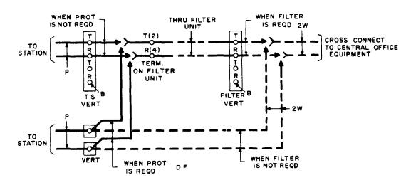
Fig. 34 - Method of Showing Optional Wiring
