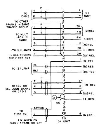
Fig. 4 — Terminations Shown at Ends of Leads (224-type terminal strip shown)
