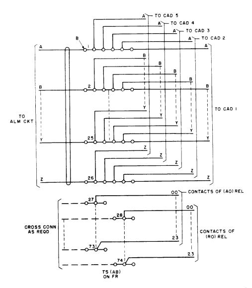
Fig. 11 - Method of Showing Clip-Type Terminals (66B5-37 Connecting Block shown)
