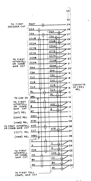
Fig. 29 — Switchboard Cable Run Direct to Relay
