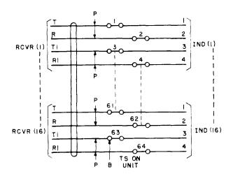
Fig. 12 – Terminal Assignment for Clip-Type
