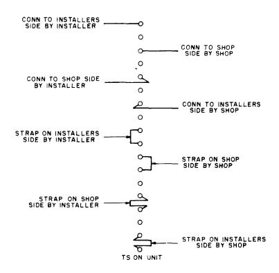
Fig. 1 - Method of Showing Shop and Installer Wiring on Terminal Strips
