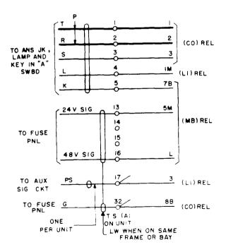
Fig. 18 – Terminal Assignment on 224-Type
