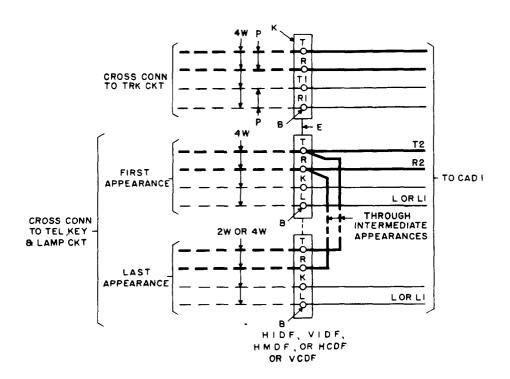
Fig. 10 – Distributing Frame Terminal Strips
