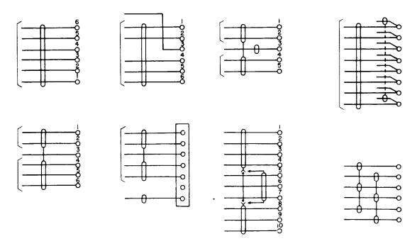
Fig. 28 - Method of Showing Cables or Wire Run on Cable Rack
