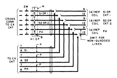
Fig. 2 - Method of Showing Cross Connections or Direct Cabling
