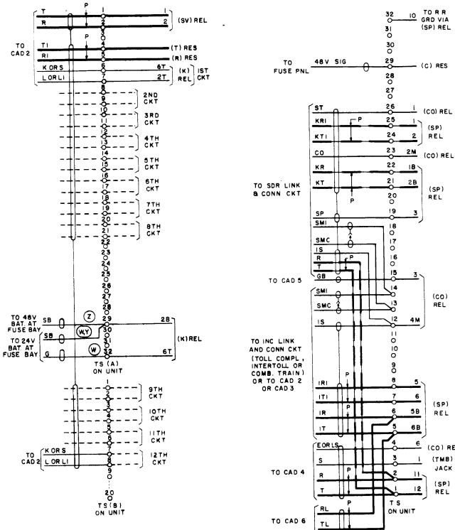
Fig. 8 - Terminals Numbered From Top to Bottom (224-type terminal strip shown)
