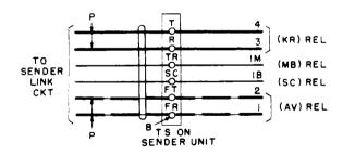
Fig. 3 — Conventions For Talking, Signaling, Etc, Leads
