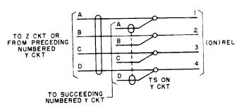
Fig. 31 — Method of Showing Leads Multipled in Numerical Sequence
