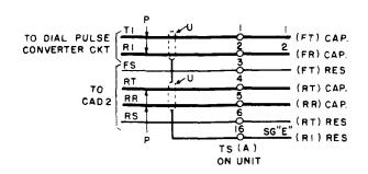
Fig. 7 - Method of Showing Shielding (203-type terminal strip shown)
