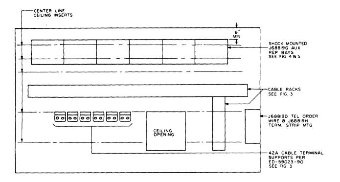
Fig. 2-Typical Layout of an Underground Auxiliary Repeater Station
