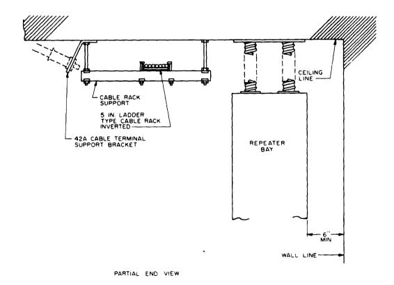
Fig. 3----Typical Cable Rack Arrangement
