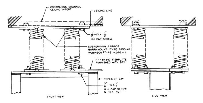
Fig. 5—Fastening Shock Mount System
