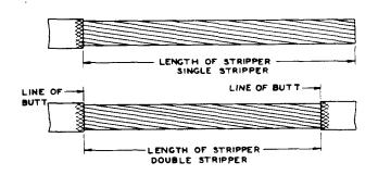
Fig. 1—Single and Double Strippers
