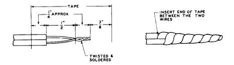
Fig 3—End Splice for Individual Conductors
