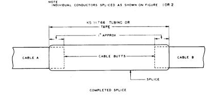
Fig 7—Straight Splice for Switchboard and Lead-Covered Cables
