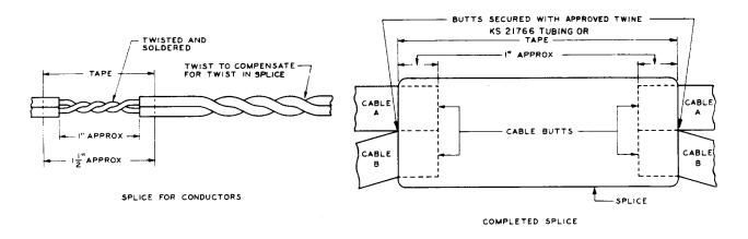
Fig 10—X Splice for Switchboard and Lead-Covered Cables
