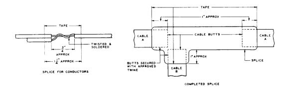
Fig 8-T Splice for Switchboard and Lead-Covered Cables
