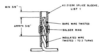
Fig 5—KS-21256 Splice Sleeve Used for Splicing 28and 30-Gauge Conductors (Sleeve Shown Cross Sectioned and Not Shrunk)
