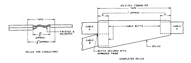
Fig 9—Y Splice for Switchboard and Lead-Covered Cables
