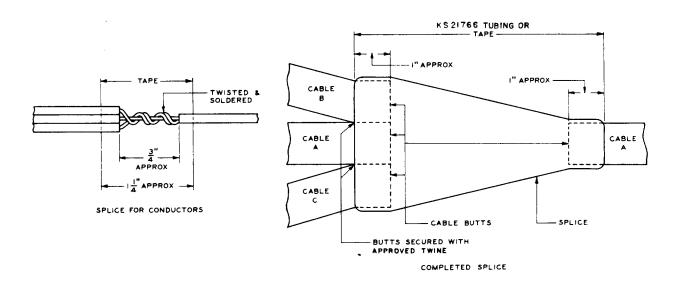
Fig 11—YY Splice for Switchboard and Lead-Covered Cables
