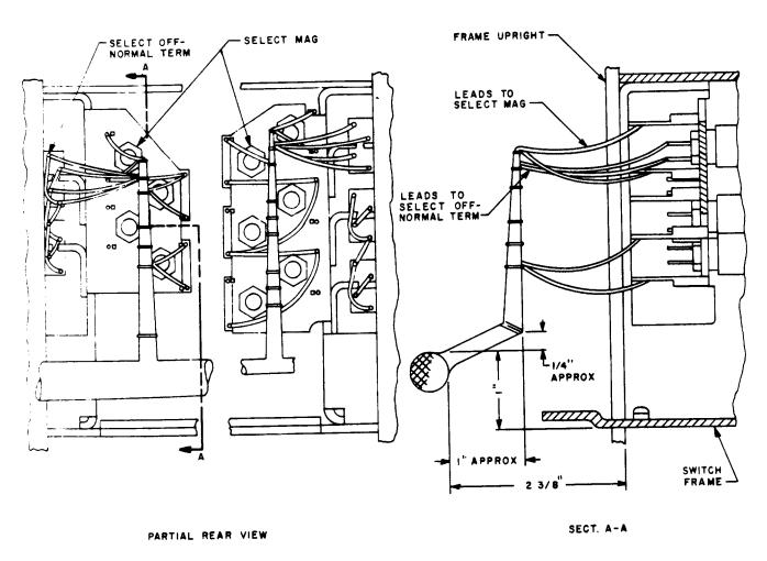
Fig. 34A—CA to CF and Similar Type Switches—Selecting Magnets and Selecting Off-Normal Spring Terminals
