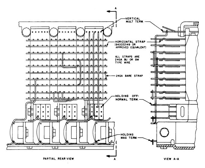
Fig. 34C—CA to CF and Similar Type Switches—Strapping of Vertical Units
