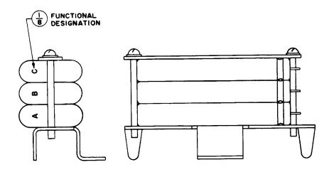
Fig. 15 – Capacitors – Mounted on 49A Bracket on Step-by-Step Switch Unit Mounting Plates
