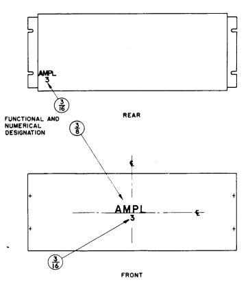
Fig. 1 – Typical Apparatus Coded Panel Assembly
