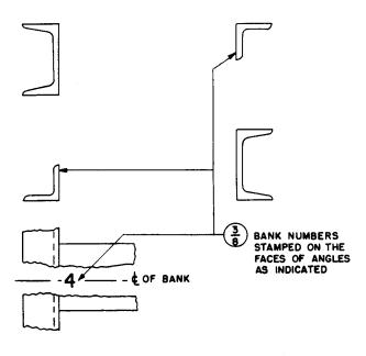
Fig. 3 – Multiple Bank Numbers When Stamped on the Framework
