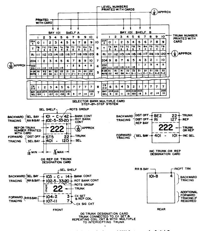
Fig. 27 – Designation Cards for Step-by-Step and PBX Systems – the Switch-Type Designation Cards Illustrated Are For Trunks and Repeaters Only
