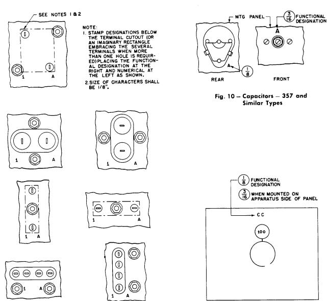
Fig. 9 – Capacitors – 227 and Similar Types – Stud Mounted Fig. 11 – Capacitors – 436 and Similar Types
