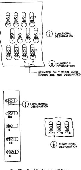
Fig. 25 – Cord Fasteners – 9 Type – Not on Cord Shelves
