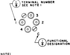
1. REGARDLESS OF THE ROTATION OF THE CAPACITOR MOUNTING, THE TERMINAL NUMBER SHALL BE LOCATED ADJACENT AND ON A HORIZONTAL LINE WITH THE ASSOCIATED TERMINAL.
