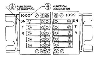
Fig. 23 - Connecting Block - 50 Type
