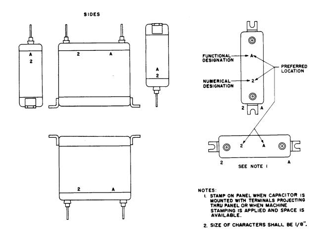
Fig. 5 – Capacitors – 170 and Similar Types – Lug Mounted
