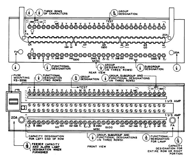
Fig. 7 – Dial Frame Fuse Panel — Double-Row Common Bus Bar —
