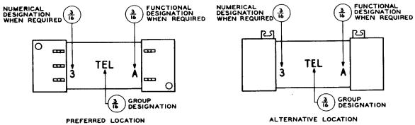
Fig. 42 - Induction Coils - 62, 63, 75A, 178, and Similar Types
