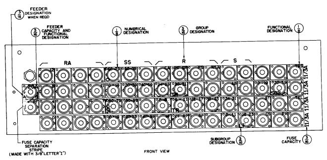
Fig. 20 – Dial Frame Fuse Panel — One Feeder — More Than Three Groups —
