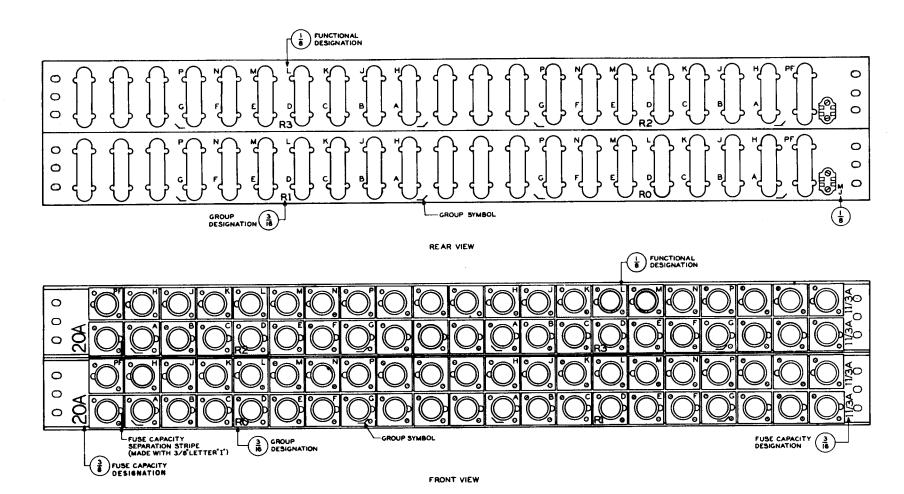
Fig. 15 – Dial Frame Fuse Panel — Two Mounting Plates — Two Feeders —
