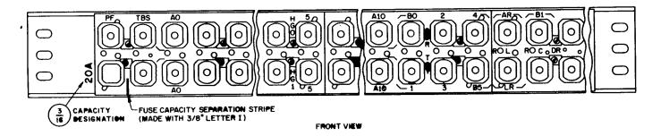
Fig. 29 — Dial Frame Fuse Panel — 22- or 23-Type Fuse Blocks Mounted on 245C and Similar Type Mounting Plates With Intermediate Cutouts — One Voltage
