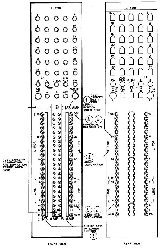
Fig. 12 – Dial Shelf Fuse Panel — Double Row With Common Bus Bar — Mounted Vertically
