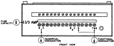
Fig. 5 – Dial Frame Fuse Panel — Single Row With Common Bus Bar — No Feeder Fuse
