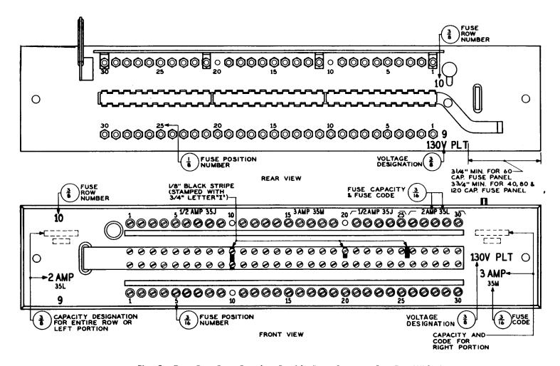
Fig. 3 — Fuse Bay Fuse Panel — Double-Row Common Bus Bar With Fuse Record Book
