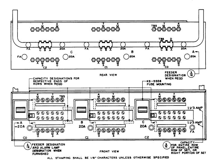
Fig. 9 – Dial Frame Fuse Panel — Double Row With Three Common Bus Bars —
