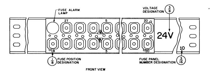
Fig. 26 — Fuse Bay Fuse Panel — Typical Stamping of 22- or 23-Type Fuse Blocks When Fuse Record Book Is Provided — 70-Type Fuses
