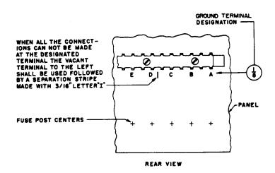
Fig. 24 — Method of Stamping Ground Terminals on Fuse Panels
