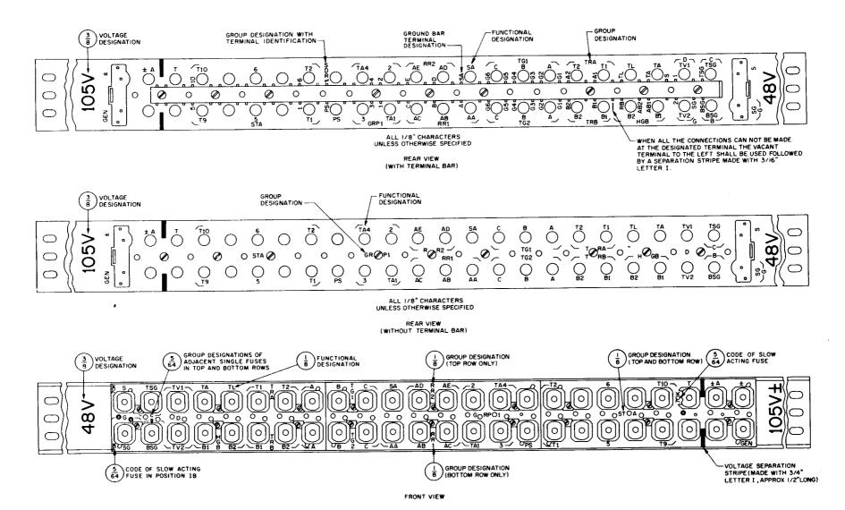
Fig. 27 – Fuse Bay Fuse Panel Without Fuse Record Book or Dial Frame Fuse Panel — Typical Designations on 22- or 23-Type Fuse Blocks — 70-Type, Fuses — Two Voltages
