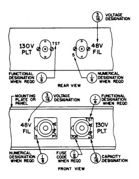
Fig. 25 — 70-Type Fuses Individually Mounted on Mounting Plate or Panel (21-type fuse block shown)
