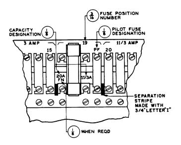
Fig. 35 - Cartridge-Type Fuse and Pilot Fuse Mounted on Fuse Panel
