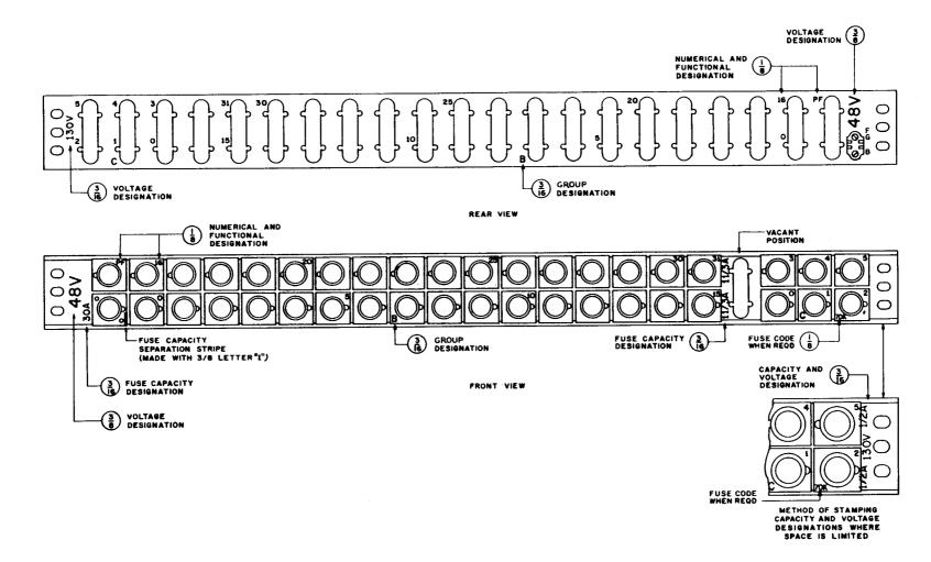
Fig. 17 – Dial Frame Fuse Panel — One Feeder — Two Voltages — Using 70-Type Fuses With 18- or 21-Type Fuse Blocks (21-type shown) and Bussman Type AGS Fuses With 20-Type Fuse Blocks
