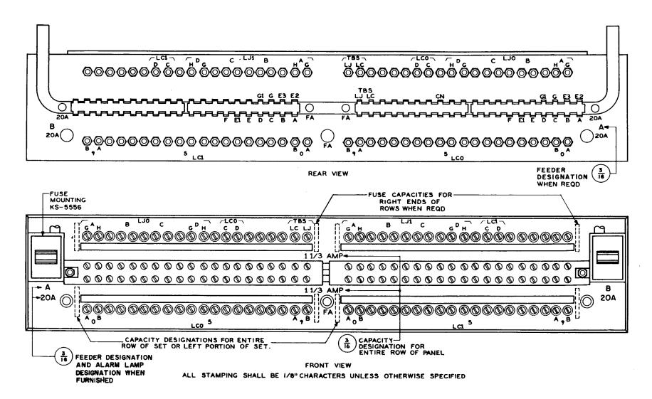
Fig. 8 – Dial Frame Fuse Panel — Double Row With Two Common Bus Bars —
