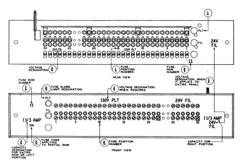
Fig. 2 – Fuse Bay Fuse Panel — Single Row Individually Mounted With Fuse Record Book
