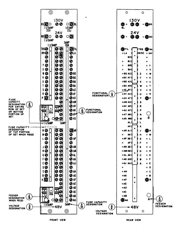
Fig. 13 – Dial Frame Fuse Panel — Double Row With Common Bus Bar — Mounted Vertically
