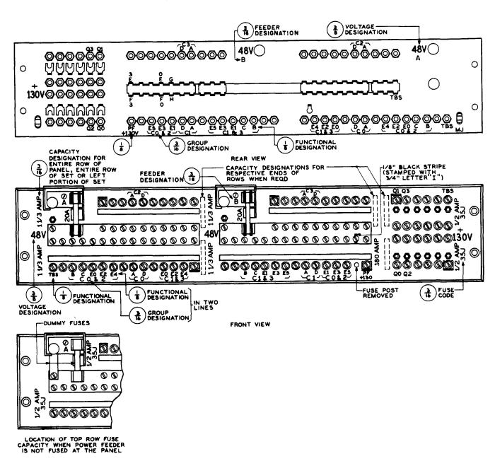
Fig. 6 - Dial Frame Fuse Panel — Double Row With Two Common Bus Bars — Two Feeders With Cartridge Fuses
