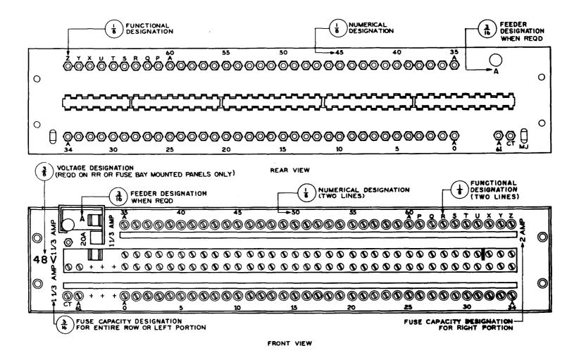
Fig. 10 – Dial Frame Fuse Panel — Double Row With Common Bus Bar — One Feeder and Cartridge Fuse
