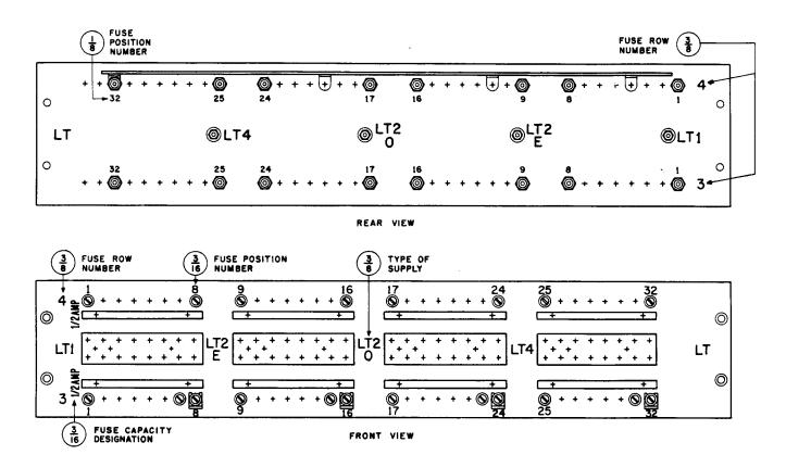
Fig. 11 - Dial Frame Fuse Panel—Less Than Ten Fuses Per Row in Each Section With Fuse Record Book
