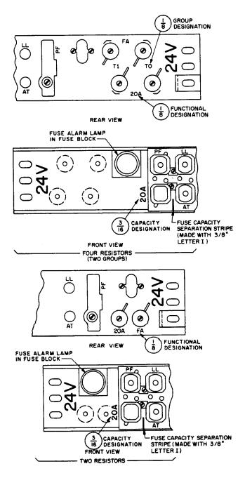
Fig. 31 — Dial Frame Fuse Panel — 20-Ampere Fuse and 70-Type Pilot Fuse in 22- or 23-Type Fuse Block — Resistors and Lamp Associated With Fuse Alarm Circuit
