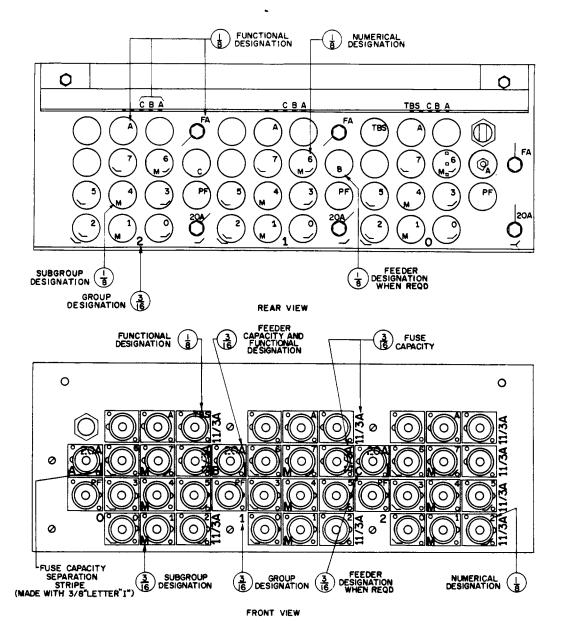
Fig. 19 – Dial Frame Fuse Panel — Three Feeders — Three Groups — Using 70-Type Fuses With 18-Type Fuse Blocks and Bussman Type AGS Fuses With 20-Type Fuse Blocks
