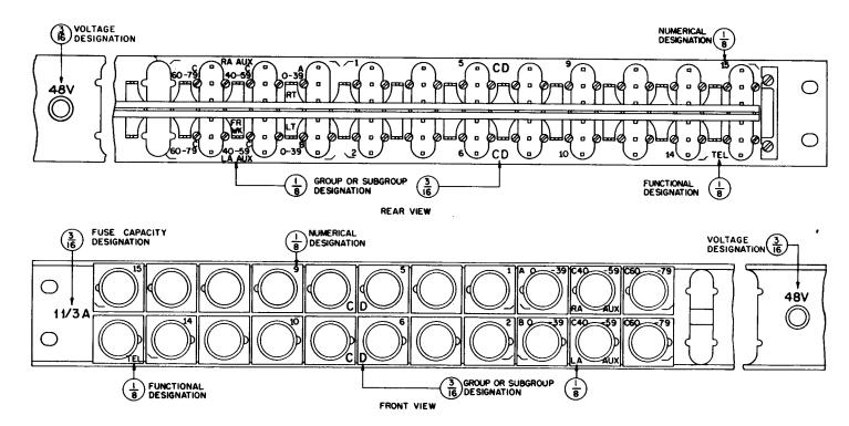
Fig. 23 - PBX Fuse Panel — One Voltage — Using 70-Type Fuses (21-type fuse blocks shown)
