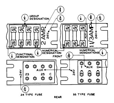
Fig. 36 - Fuses on 606-Type Mounting Plates
