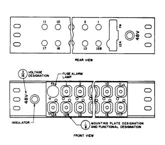
Fig. 30 – PBX Fuse Panel — Fuse Alarm Lamp and 70-Type Fuses in 22- or 23-Type Fuse Blocks — One Voltage
