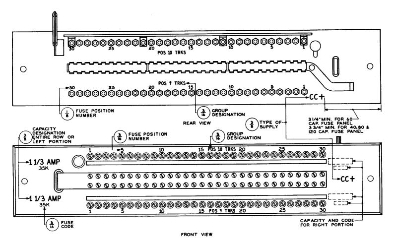
Fig. 4 – Fuse Bay Fuse Panel — Double-Row Common Bus Bar Without Fuse Record Book
