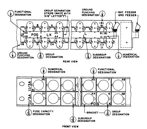
Fig. 21 – Dial Frame Fuse Panel — One Voltage — Using 70-Type Fuses (21-type fuse blocks shown)
