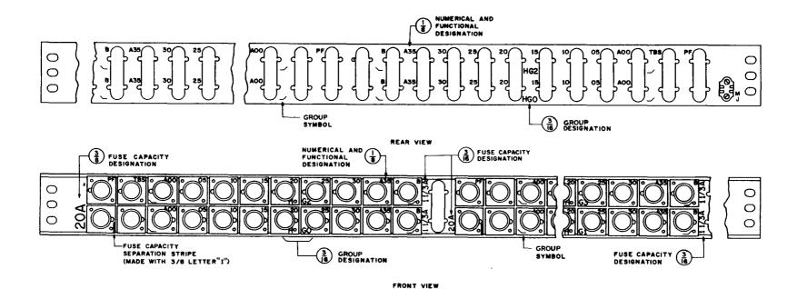
Fig. 16 – Dial Frame Fuse Panel — Two Feeders — Four Subgroups — Using 70-Type Fuses With 18-Type Fuse Blocks and Bussman Type AGS Fuses With 20-Type Fuse Blocks
