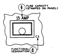
Fig. 37 - KS-5780 Fuse Mounting
