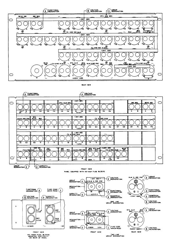
Fig. 32 - Panel Equipped With KS-14169 Fuse Blocks
