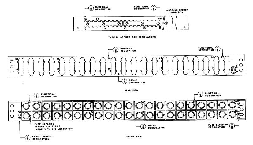
Fig. 18 – Dial Frame Fuse Panel — One Feeder — Using 70-Type Fuses With 18-Type Fuse Blocks and Bussman Type AGS Fuses With 20-Type Fuse Blocks
