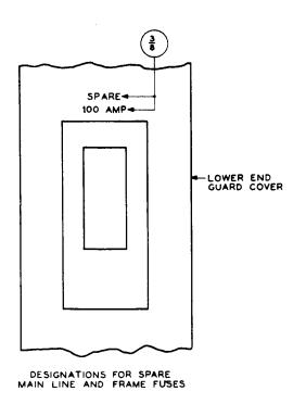
Fig. 41 – Designations for Spare Main Line and Frame Fuses
