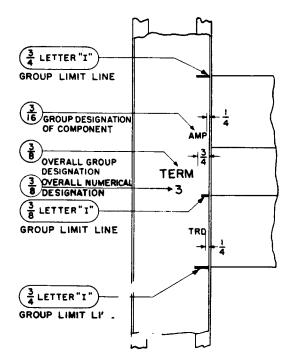
Fig. 12 - Group Designations for Components Included in a Set of Components Requiring Over-all Group Designation for the Set -Closed-duct Side of Single-sided Bay
