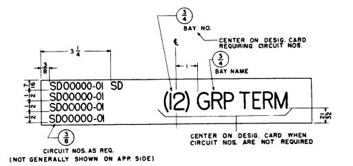
Fig. 7 - Designations on Bay Designation Card -Auxiliary Framing Supported Bays
