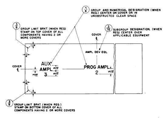
Fig. 2 - Designations on Panel Cover - Open-duct or Closed-duct Side
