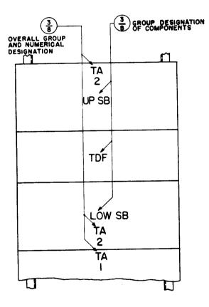
Fig. 5 - Over-all Designation for Group of Components (Less Than Complete Bay)
