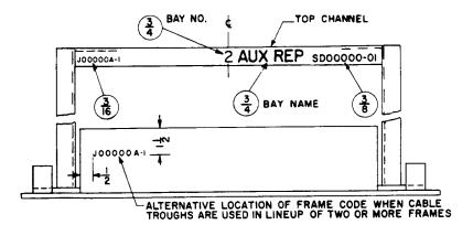
Fig. 9 - Bay Name, Bay Number, SD Drawing Number and J Code Stamping on 6-foot 0-inch and 7-foot 0-inch Floor-supported Bay Framework
