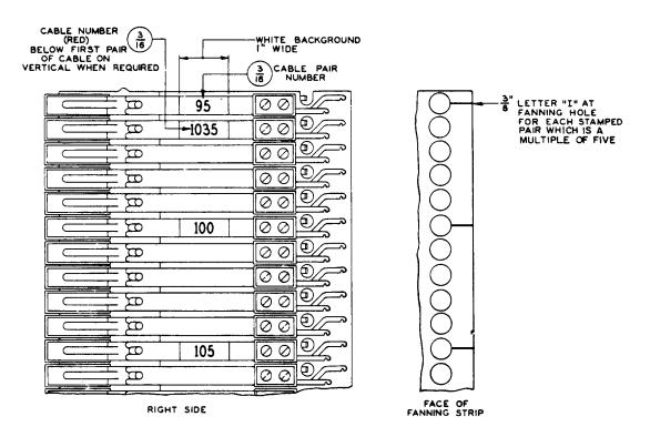
Fig. 2 – Protectors When Designations for Loading, etc, Are Not Required — MDF, CDF, and Protector Frames
