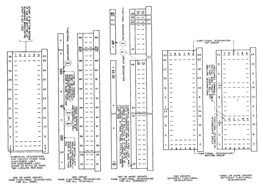
Fig. 41 – Terminal Sirips — Functional and Numerical Designations — Two or More Circuits per Row
