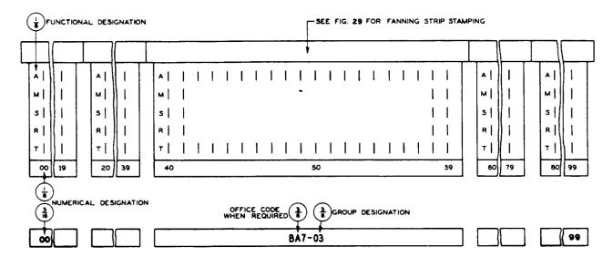
Fig. 31 – Terminal Strips — 178AA, 178AF, 178AG, or Similar Types — Subscriber Lines — Panel and Step-by-Step IDF
