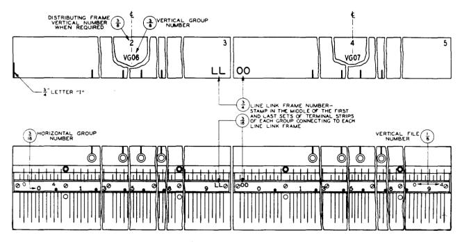
Fig. 14 – Terminal Strips — 182 and Similar Types — Subscriber Lines, Tip and Ring Leads — No. 5 Crossbar MDF
