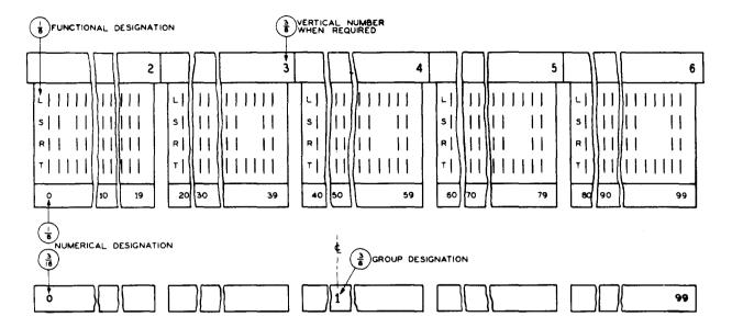
Fig. 9 – Terminal Strips — 150AE, 150AJ, and Similar Types — Subscriber Lines — Manual MDF and CDF
