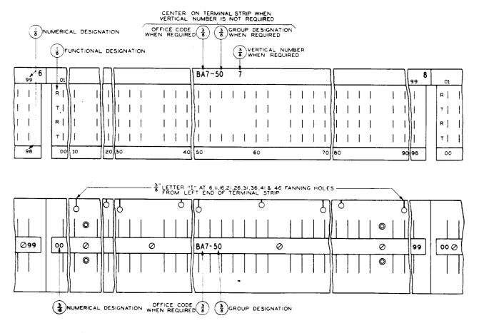
Fig. 12 – Terminal Strips — 183 and Similar Types — Subscriber Lines — Panel and No. 1 Crossbar MDF
