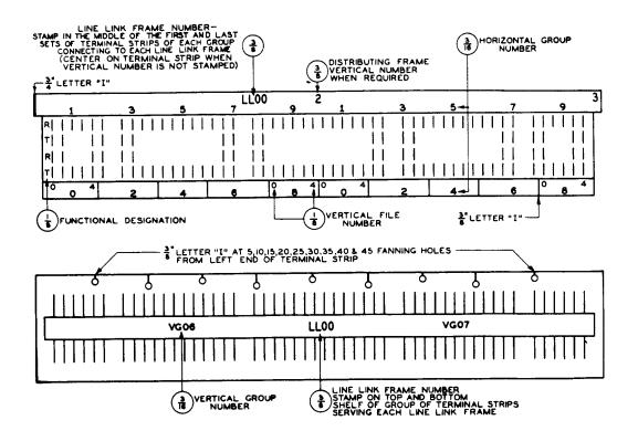
Fig. 16—Terminal Strips — 183 and Similar Types — Subscriber Lines,
