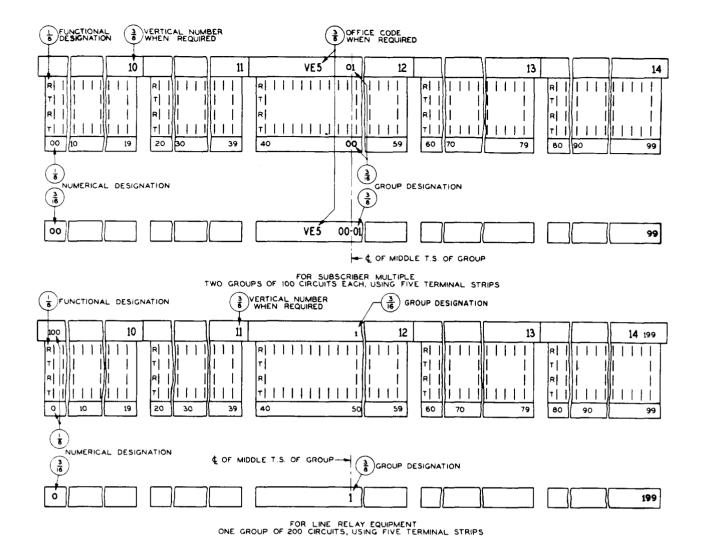
Fig. 13 – Terminal Strips — 231 and Similar Types — Subscriber Lines — Panel and No. 1 Crossbar MDF
