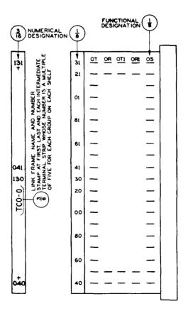
Fig. 35 - Terminal Strips — Link Frame
