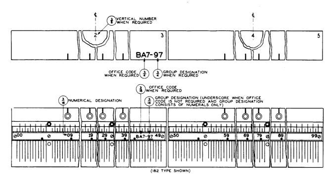
Fig. 11 – Terminal Strips — 65, 182, and Similar Types — Subscriber Lines — Panel, Step by Step, PBX, and No. 1 Crossbar MDF
