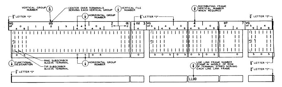
Fig. 20 — Terminal Strips — 183 and Similar Types — Subscriber Lines, Sleeve Leads (Two Terminals per Circuit) — No. 5 Crossbar MDF
