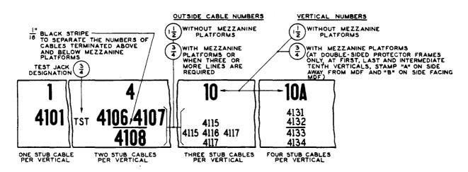
Fig. 1 - Cable Designation Boards - MDF, CDF, and Protector Frames
