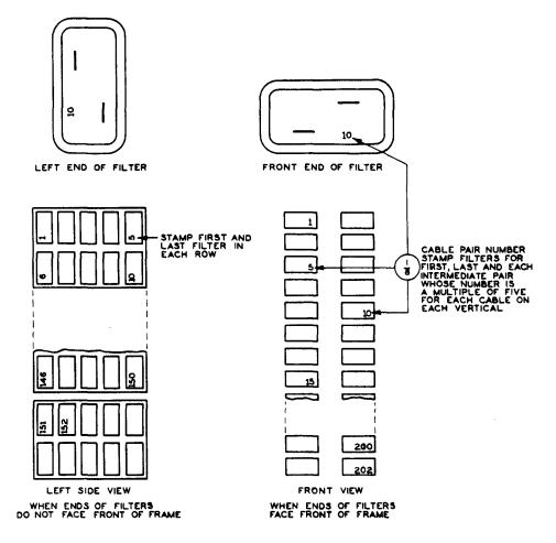
Fig. 23 - Filters on Distributing Frames
