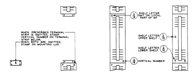
Fig. 26 – Frame Vertical Numbers and Shelf Letters — Vertical Side — Toll IDF, Double-sided TDF, TADF, TRDF, CDF Not Equipped With Cable Designation Board, and Local Part of an IDF Serving Both Local and Toll
