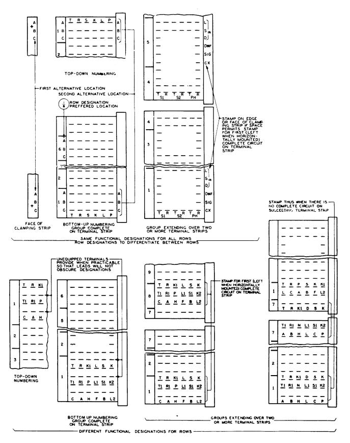
Fig. 44 – Terminal Strips — Functional and Numerical Designations —
