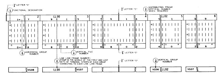
Fig. 15 – Terminal Strips — 231 and Similar Types — Subscriber Lines, Tip and Ring Leads — No. 5 Crossbar MDF
