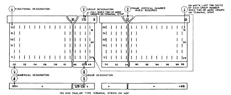
Fig. 34 -Terminal Strips — Subscriber Lines — LDF and LDF Equipment on MDF
