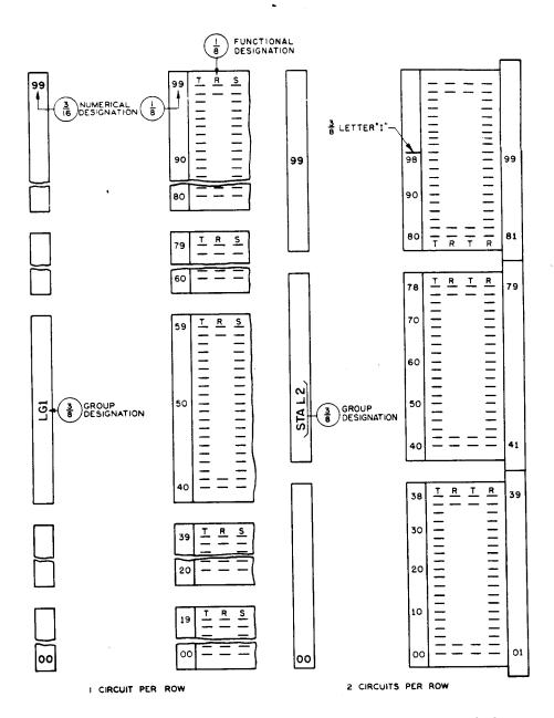
Fig. 25 – Terminal Strips — Subscriber Lines — Step-by-Step CDF
