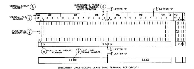
Fig. 18 — Terminal Strips — 183 and Similar Types — Subscriber Lines, Sleeve Leads (One Terminal per Circuit) — No. 5 Crossbar MDF
