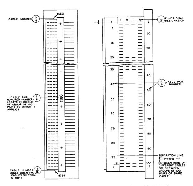
Fig. 6 – Terminal Strips — For Cable Pairs of Outside Cables and for Tie Cables
