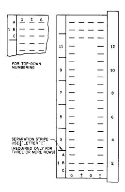
Fig. 42 - Terminal Strips — Functional and Numerical Designations — Two or More Circuits per Two or More Rows
