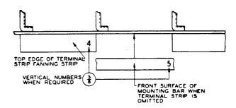
Fig. 8 — Vertical Numbers on Top Edge of Horizontal Terminal Strips — MDF, Double-sided CDF, and TDF
