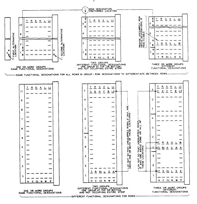
Fig. 43 — Terminal Strips — Functional and Numerical Designations —
