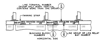
Fig. 29 - Designations Applying to Equipment on Opposite Vertical — Panel and Step-by-Step IDF
