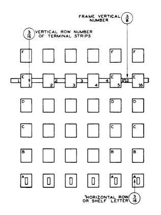
Fig. 30 — Frame Vertical and Terminal Strip Vertical
