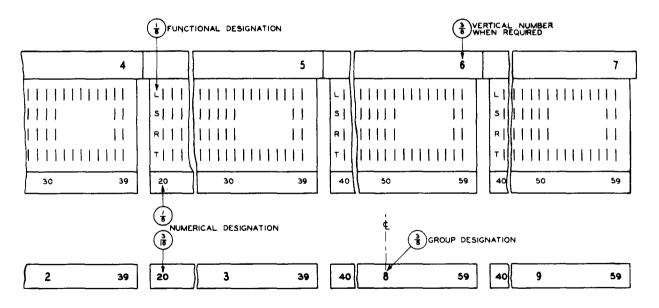
Fig. 10 – Terminal Strips — 178AB and Similar Types — Subscriber Lines — No. 12 Manual MDF
