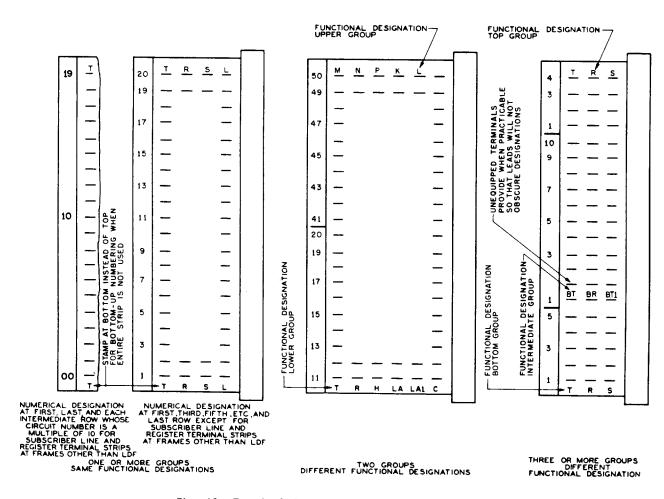
Fig. 40 – Terminal Strips — Functional and Numerical Designations — One Circuit per Row
