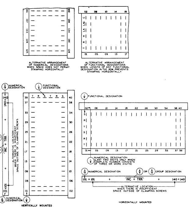
Fig. 37 - Terminal Strips - General Requirements for Size and **Orientation of Characters**
