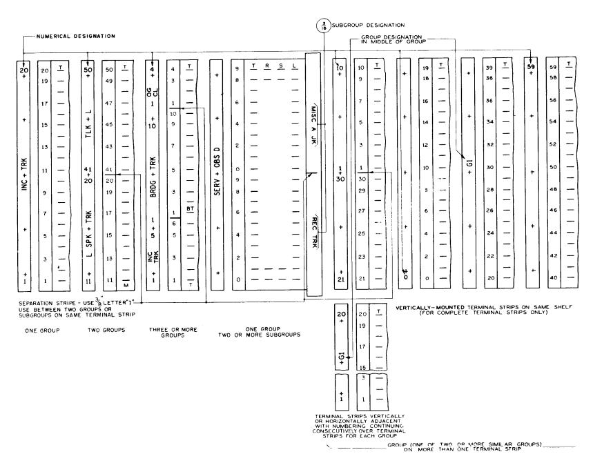
Fig. 38 – Terminal Strips — Group Designations and Use of Numerical Designations and Group Separation Stripes Therewith
