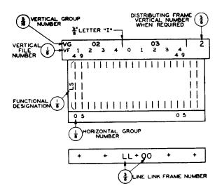
Fig. 17 – Terminal Strips — 268C and Similar Types — Subscriber Lines, Sleeve Leads (One Terminal per Circuit) — No. 5 Crossbar MDF
