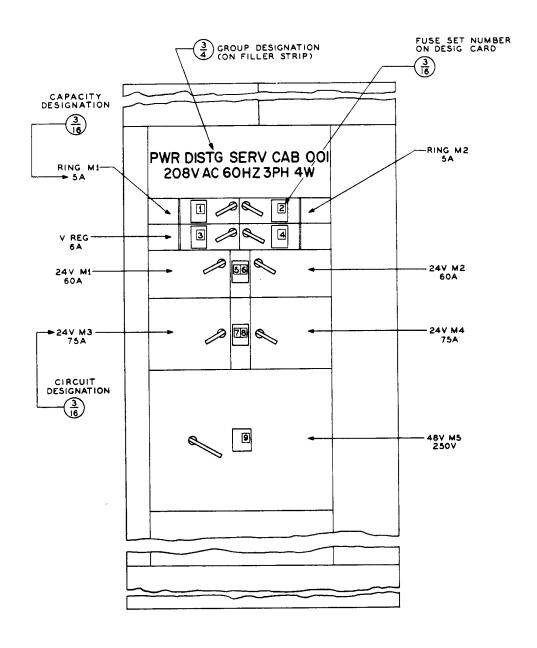
Fig. 31 - Power Distributing Service Switch and Fuse Switchboard - KS-15699 Type
