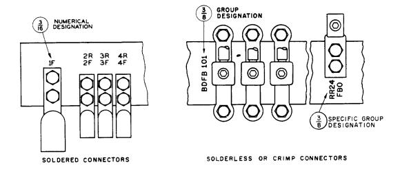
Fig. 14 - Ground Bus Bar at Power Board
