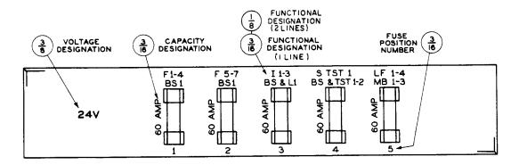
Fig. 25 - Cartridge-Type Fuse Panel
