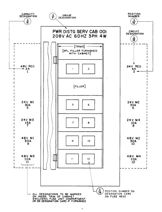
Fig. 30 - Power Distributing Service Fuse Cabinet - Wall-Mounted - KS-5774 or KS-15727 Type
