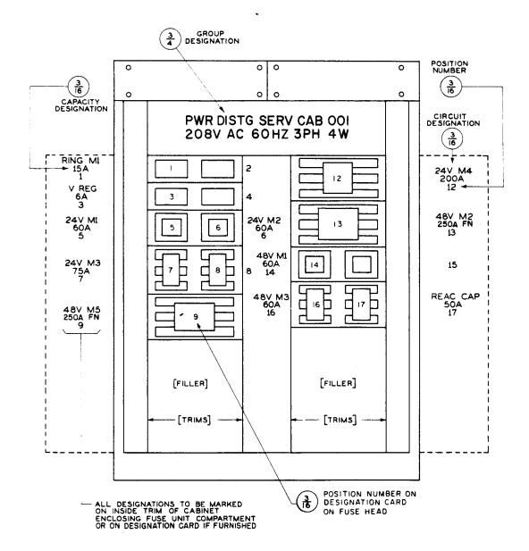
Fig. 29 - Power Distributing Service Fuse Cabinet Two Bays - Floor-Mounted KS-5774 Type
