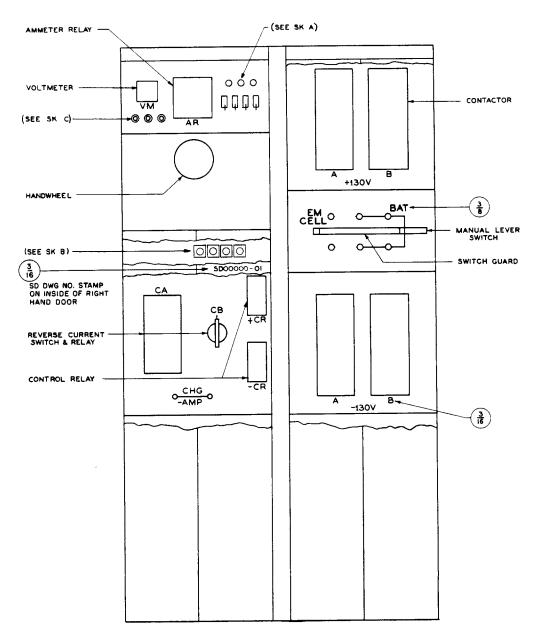
Fig. 51 - Typical Generator Control Switchboard - 2 Bays
