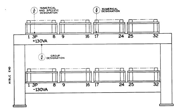
Fig. 9 - Storage Cells in Boxes or Trays on Metal Stand
