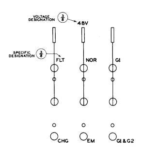
Fig. 48 - Knife Switches - Manually Operated
