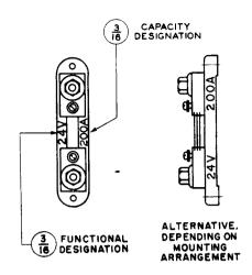
Fig. 1 - Ammeter Shunt Mounted on Block
