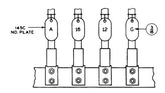
Fig. 13 - Cable Risers at Ground Bus Bar of Fuse Bays, Battery Distributing Fuseboards, MDF, CDF, or Protector Frames
