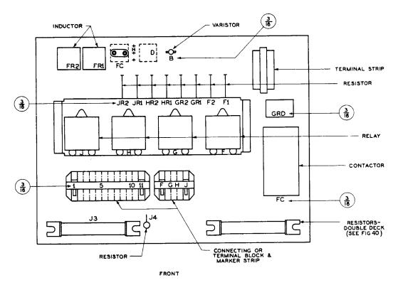
Fig. 49 - Typical Converter Panel
