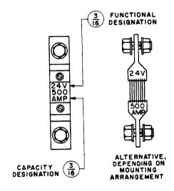
Fig. 2 - Ammeter Shunt Mounted on Bus Bars
