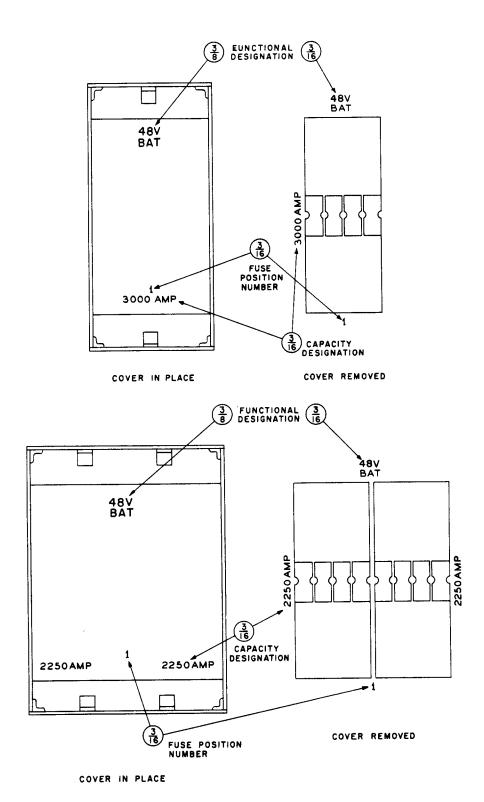
Fig. 22 - Open-Link Fuse and Enclosure
