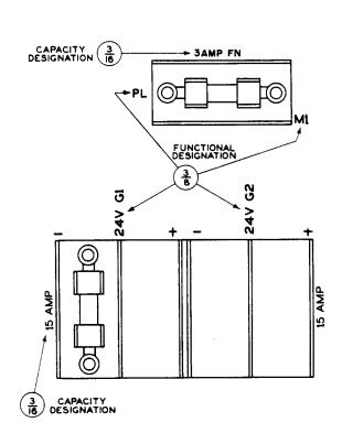
Fig. 18 - Cartridge-Type Fuses, Fusetrons, or Fustats in Fuse Holders
