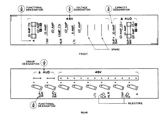
Fig. 26 - Fuse Panel With Cartridge- and Alarm-Type Fuses
