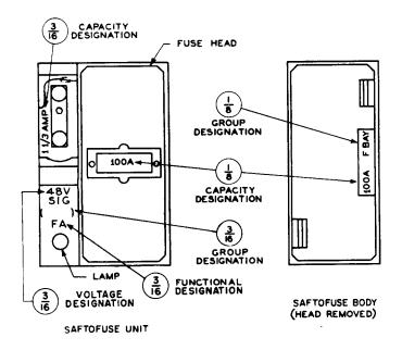
Fig. 20 - End Guard Power Fuse Mounting
