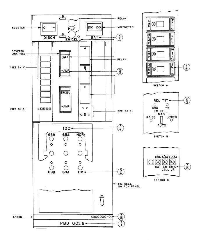
Fig. 50 - Typical Emergency Control Bay Equipment
