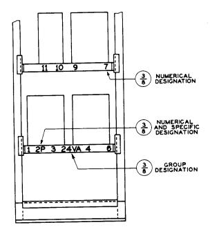
Fig. 6 - Multicell Battery Units on Relay Rack or Metal Stand
