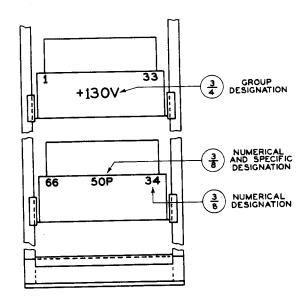
Fig. 8 - Storage Cells in Boxes or Trays on Relay Rack
