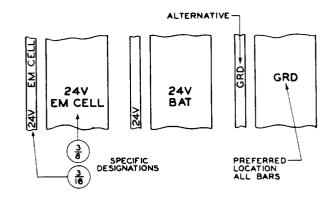
Fig. 12 - Bus Bar Risers at Emergency Cell Switch Bay
