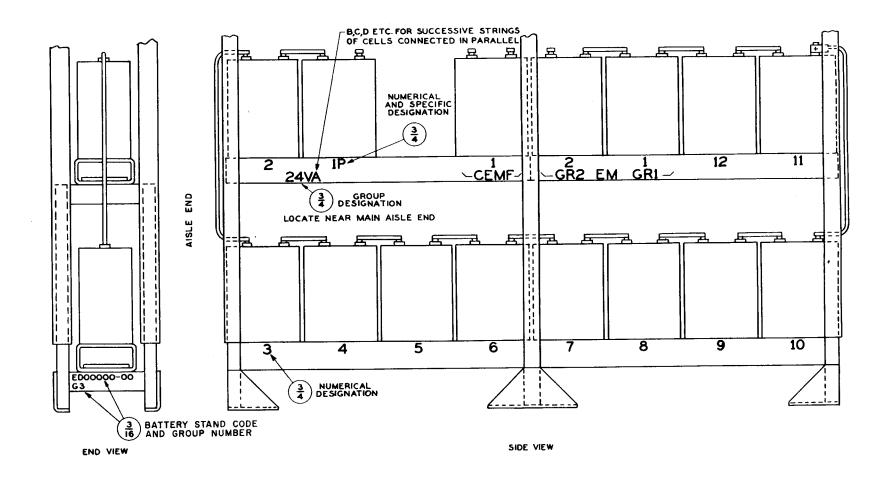
Fig. 4 - Storage Cells on Two-Tier, One-Row Stand
