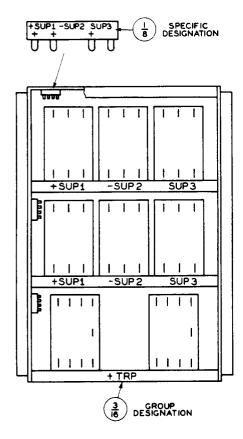
Fig. 11 - Dry Batteries - Block Type
