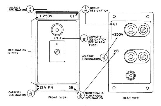
Fig. 21 - KS-14473 Fuse Mounting
