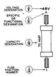
Fig. 17 - Cartridge-Type Fuse on Posts
