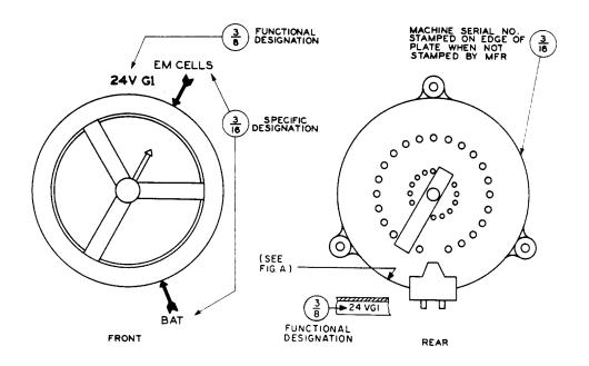
Fig. 34 - Handwheel and Field Rheostat
