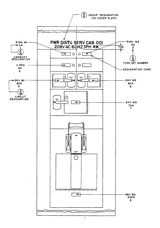
Fig. 32 - Power Distributing Service Switch and Fuse Switchboard - KS-15619 Type (A&M Only)
