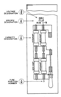
Fig. 19 - Discharge Fuses and Switch Unit
