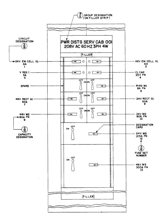
Fig. 33 - Power Distributing Service Switch and Fuse Switchboard - KS-15697 Type
