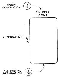
Fig. 39 - Power Relays, Bells, Contactors, or Circuit Breakers
