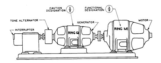
Fig. 42 - Ringing M-G Set With High- and Low-Speed Interrupters - Table Mounted
