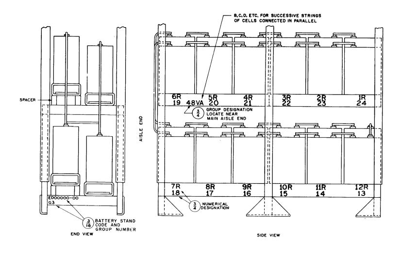
Fig. 5 - Storage Cells on Two-Tier, Two-Row Stand With One Row Per Tier on Wall Side
